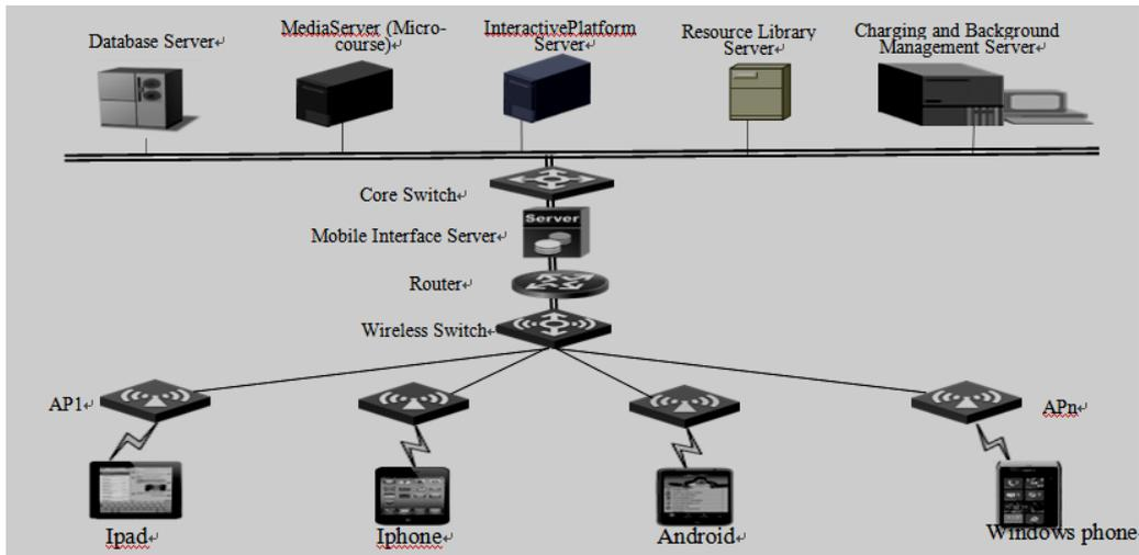
Figure 2. M-Learning Hardware Platform System Framework Topology
