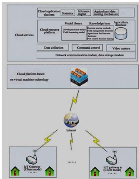
Figure 4. Cloud service platform based on virtual machine technology
