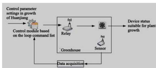
Figure 6. Strict plant environment closed-loop control system based on loop command list technology
