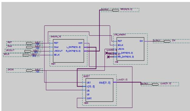
Figure 8 FPGA Implementation of Improved Logarithmic Controlled VSSLMS Algorithm.
