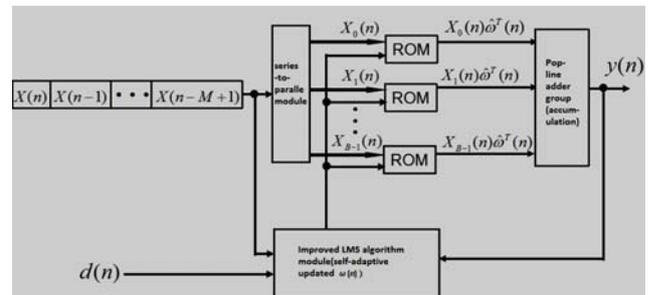
Figure 5. Hardware structure of high-speed self-adaptive fir digital filter
