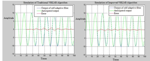
Figure 3. Comparison of traditional VSSLMS algorithm and improved VSSLMS algorithm in terms of anti-jamming capability.
