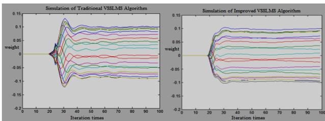
Figure 2. Comparison of VSSLMS algorithm and improved VSSLMS algorithm.
