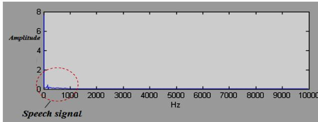
Figure 7. Frequency spectrum after filtering of voice containing noise.
