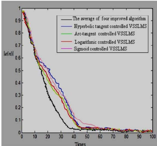
Figure 4. The comparison between the performance of the four FCVSSLMS algorithm and the average performance of their improved algorithm.
