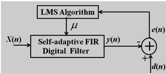
Figure 1 The structure of self-adaptive FIR digital filter based on traditional LMS algorithm.
