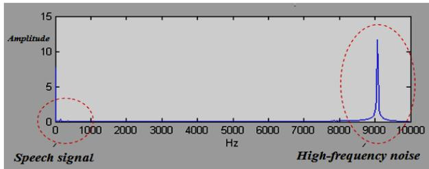
Figure 6. Frequency spectrum before filtering of voice containing noise
