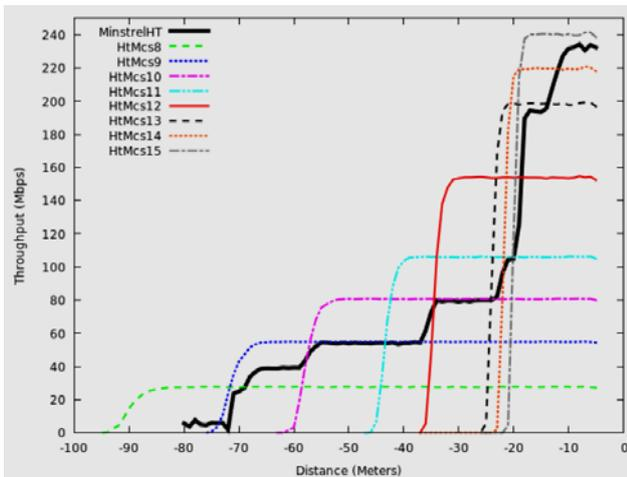
Fig. 3. Minstrel-HT performance in 802.11n WLAN with two spatial streams, the quality of non-fading channels change from bad to good.
