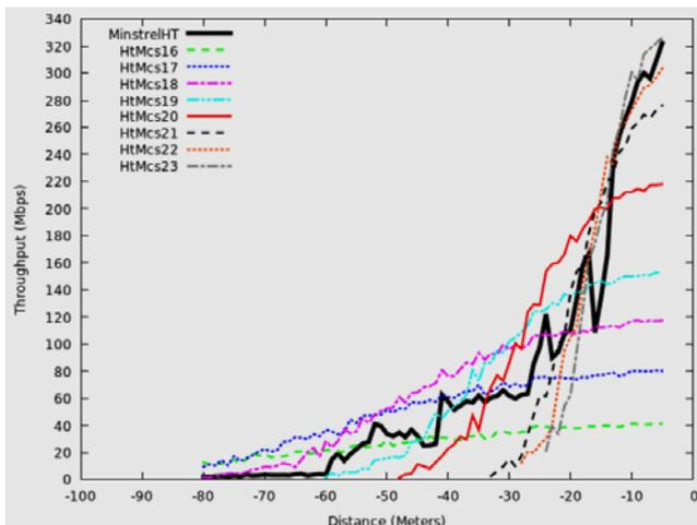
Fig. 9. Minstrel-HT performance in 802.11n WLAN with three spatial streams, the quality of fading channels change from bad to good.
