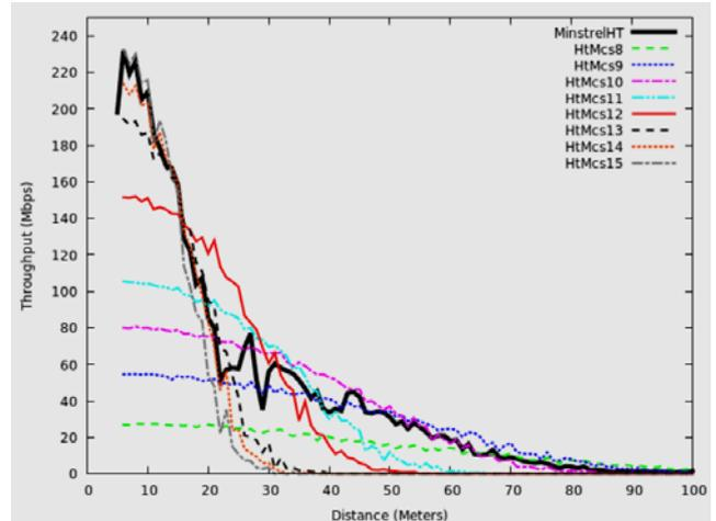
Fig. 8. Minstrel-HT performance in 802.11n WLAN with two spatial streams, the quality of fading channel change from good to bad.
