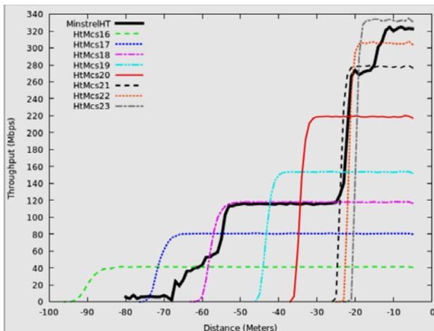
Fig. 5. Minstrel-HT performance in 802.11n WLAN with three spatial streams, the quality of non-fading channels change from bad to good.
