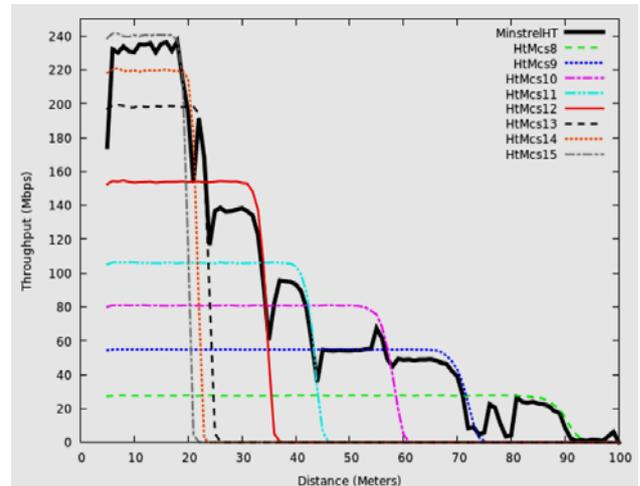
Fig. 4. Minstrel-HT performance in 802.11n WLAN with two spatial streams, the quality of non-fading channels change from good to bad.
