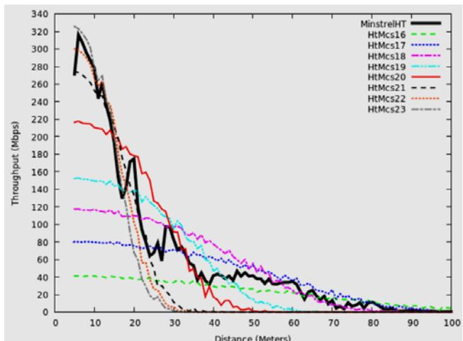
Fig. 10. Minstrel-HT performance in 802.11n WLAN with three spatial streams, the quality of fading channel change from good to bad.
