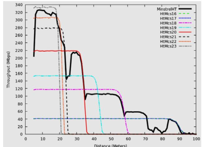
Fig. 6. Minstrel-HT performance in 802.11n WLAN with three spatial streams, the quality of non-fading channels change from good to bad.
