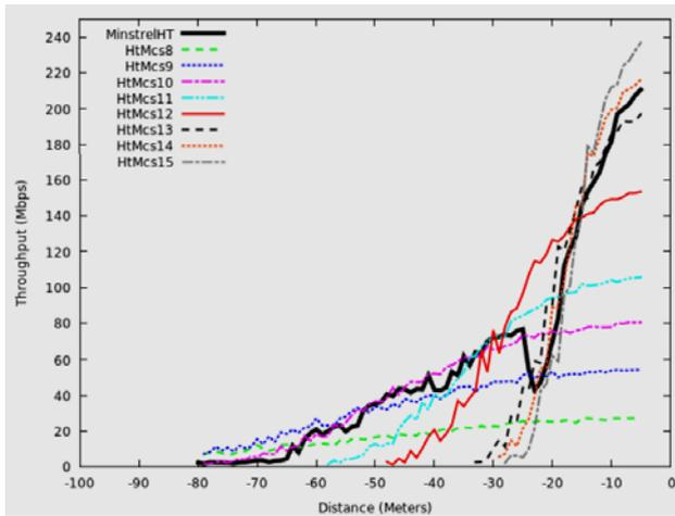
Fig. 7. Minstrel-HT performance in 802.11n WLAN with two spatial streams, the quality of fading channels change from bad to good.
