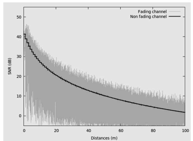
Fig. 2. 802.11n channel quality model in 40 MHz channel width
