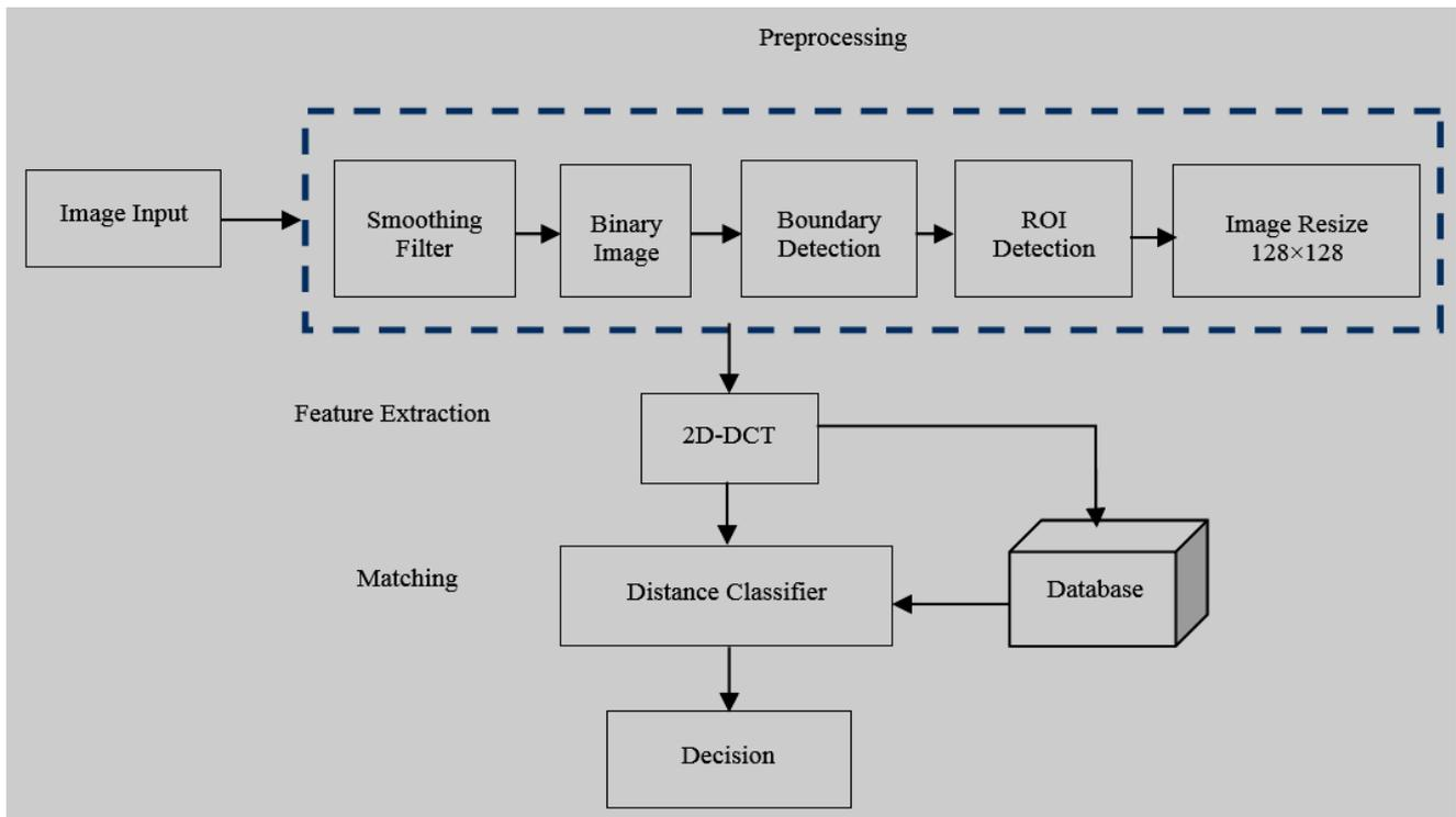
Fig.1. Block diagram of the proposed palm print based recognition system.
