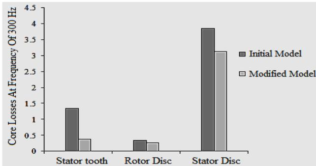
Figure 7. The core loss in frequency 300 (Hz).
