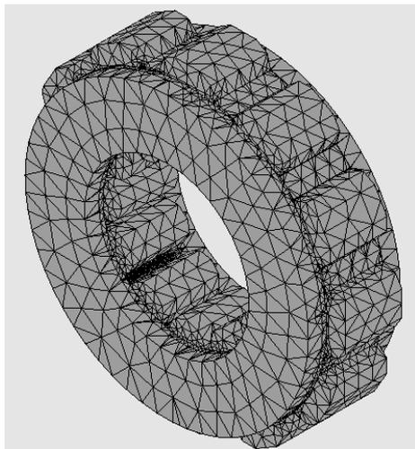
Figure 2. Finite-element mesh of the AFPM motor model.
