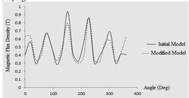
Figure 9. The comparison of air gap flux density in  $t=0.00316$  (s).
