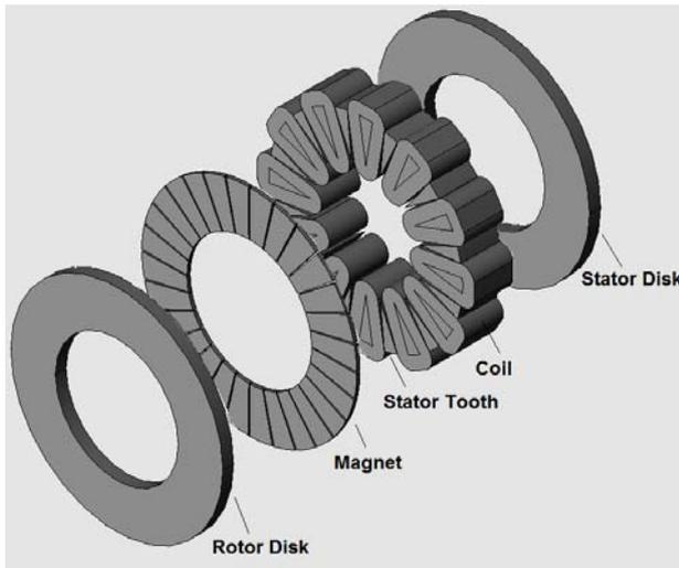
Figure 1. The analyzed AFPM motor.
