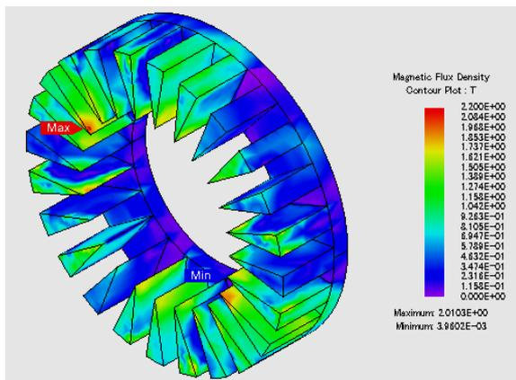
Figure 3. The flux density distribution in stator core of basic model in  $t=0.00316$  (s).
