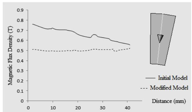
Figure 10. The comparison of air gap flux density inside magnet in  $t=0.00316$  (s).
