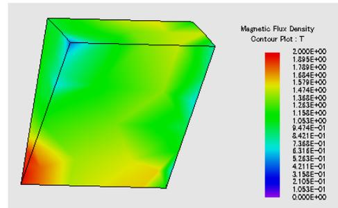
Figure 4. The flux density distribution in one stator tooth.
