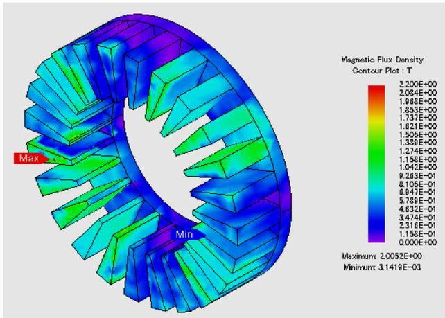
Figure 6. The flux density distribution in stator core of proposed model in  $t=0.00316$  (s).
