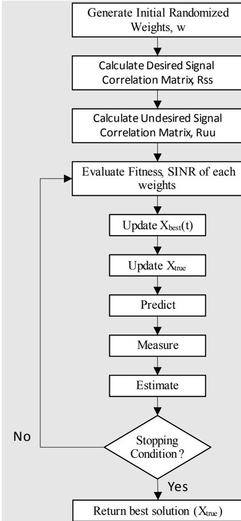
Fig. 3: The flowchart of SKF for adaptive beamforming.
