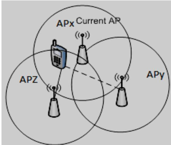
Figure 2. Example of EHP movement from APx to either APy or APz
