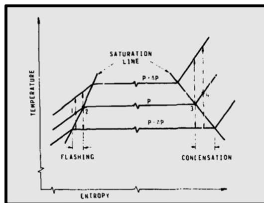
Fig. 6 temperature-entropy diagram showing spontaneous Flashing and condensation [36]
