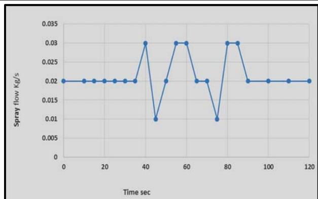
Fig.10 .spray flow optimization by genetic algorithms
