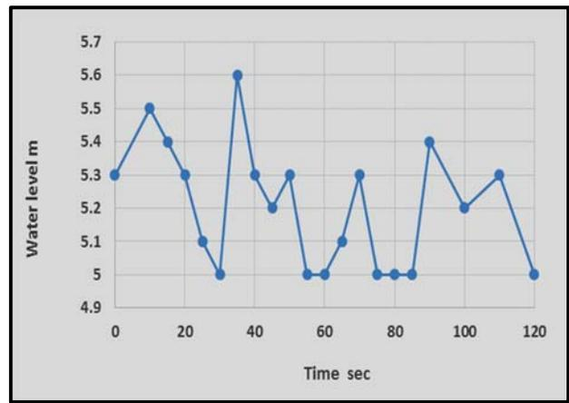
Fig. 8 .Water Level Changes during Surge Transient
