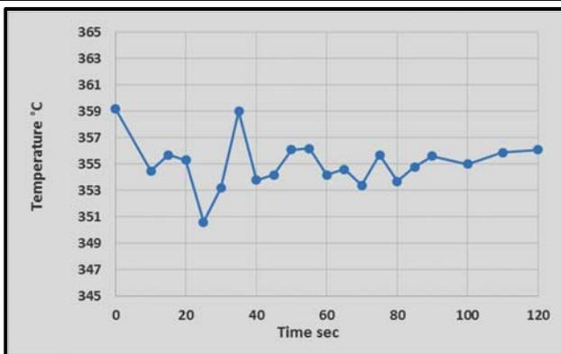
Fig. 9 .Temperature Changes during Surge Transient
