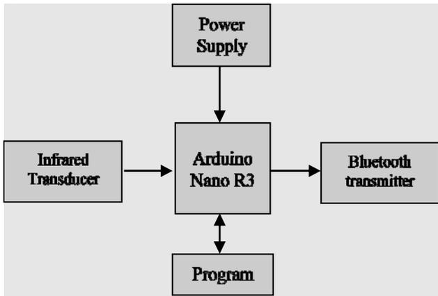
Figure 4. System interconnection for the wearable controller
