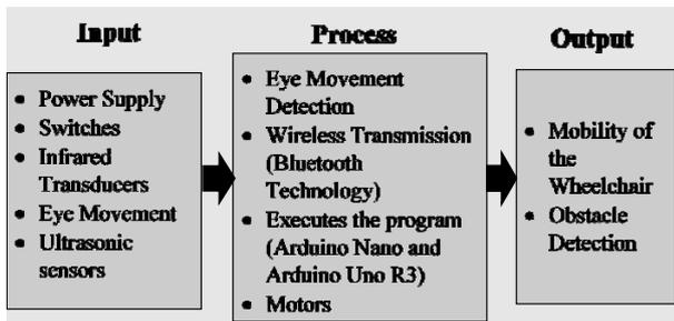
Figure 1. Block diagram showing the relationships of inputs, processes and outputs to the system
