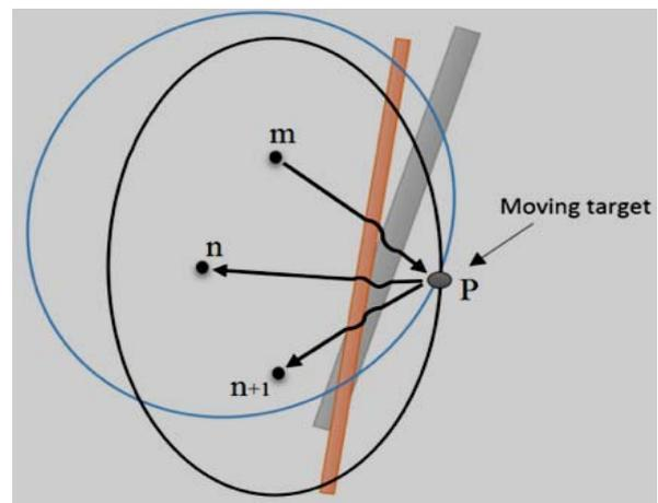
Fig. 1. Partial representation of the limited view multi-static configuration illustrating two transmitter-receiver pairs, and their corresponding ellipses.
