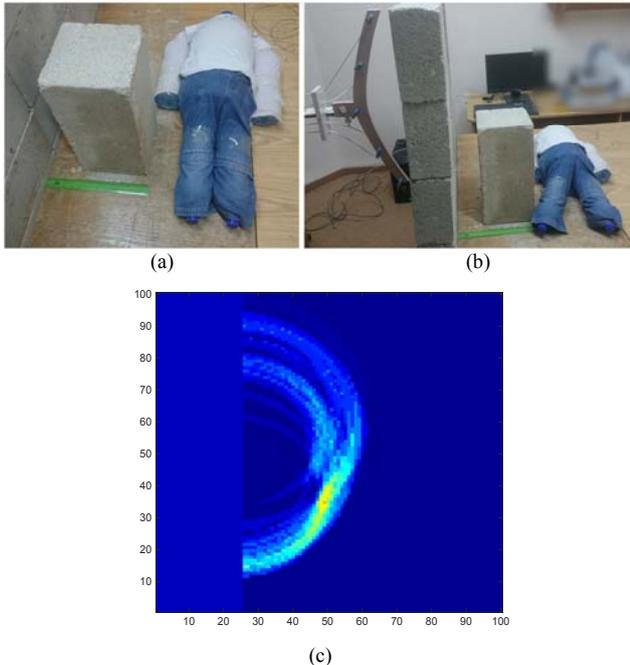
Fig 7: Detection of hand limb movement showing: (a) and (b) actual target before and after movement, and (c) the detected image
