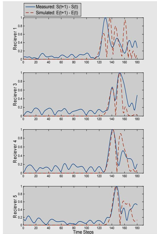
Figure 5 : Simulated and measured fields (normal magnitude) captured at receivers 1,3,4, and 5 due to the excitation of transmitter 2.
