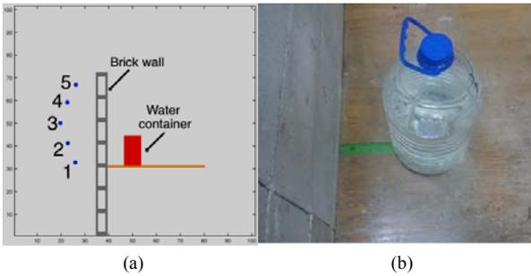
Figure 4: Simple target experiment showing: (a) simulation model, (b) actual target.
