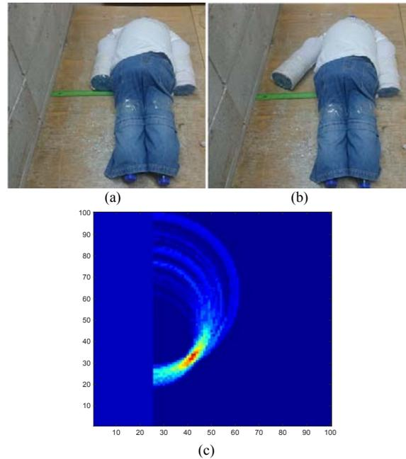
Fig 6: Detection of hand limb movement showing: (a) and (b) actual target before and after movement, and (c) the detected image
