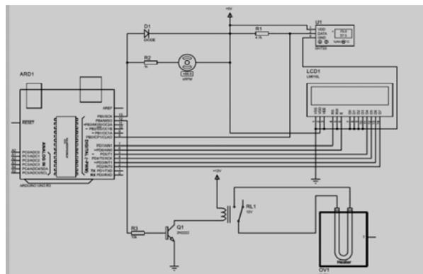
Figure 3. Circuit layout of the temperature controller using Proteus
