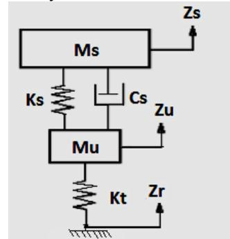
Figure 1. Passive Suspension System
