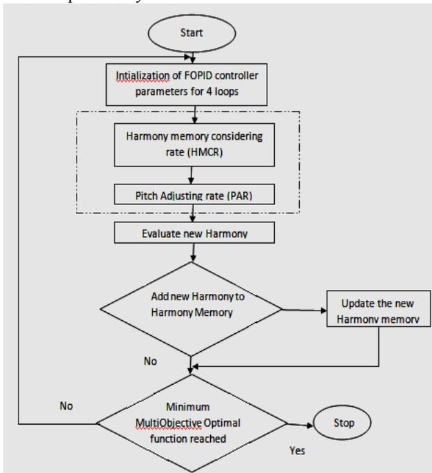
Figure 5. Flow chart of HS algorithm for FOPID controller parameter optimization
