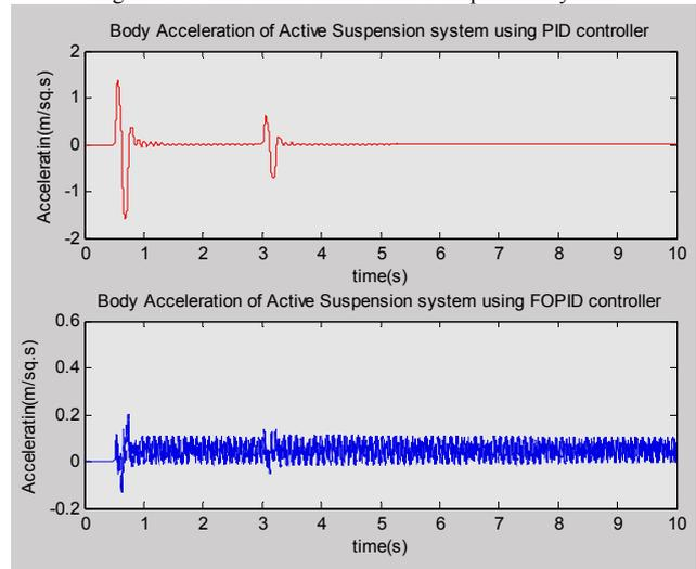
Figure 10. Body Acceleration of Active Suspension System
