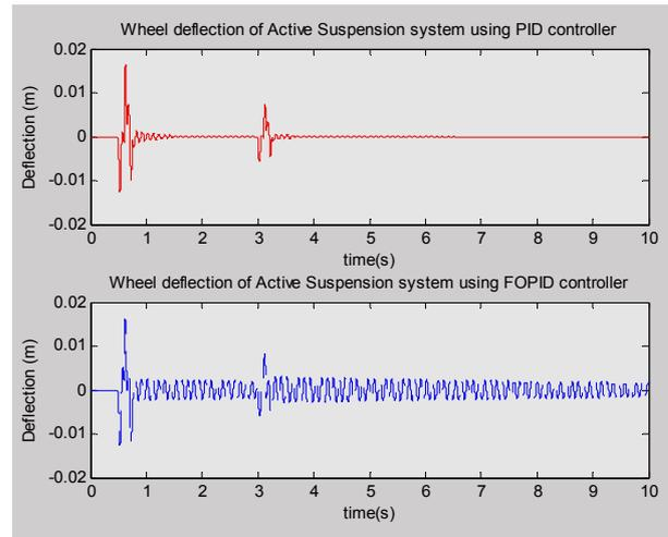
Figure 9. Wheel deflection of Active Suspension System
