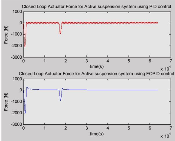
Figure 7. Actuator force for Active Suspension system.
