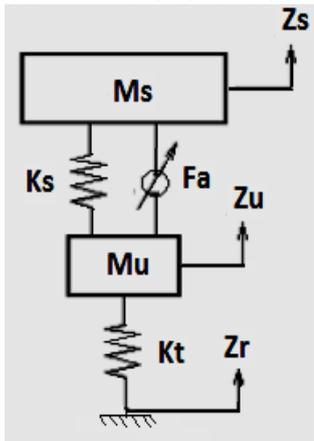
Figure 2. Active Suspension System
