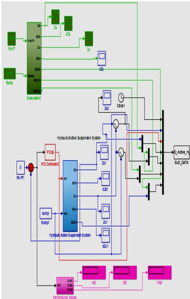
Figure 4. SIMULINK block diagram of passive and Active Suspension system.
