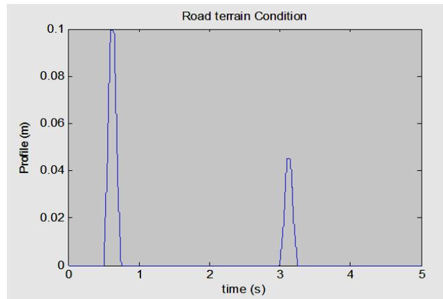
Figure 3. Road terrain Condition with two bumps.
