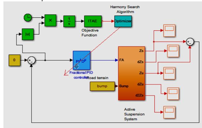
Figure 6. Harmony search algorithm optimized FOPID controller for active suspension system.
