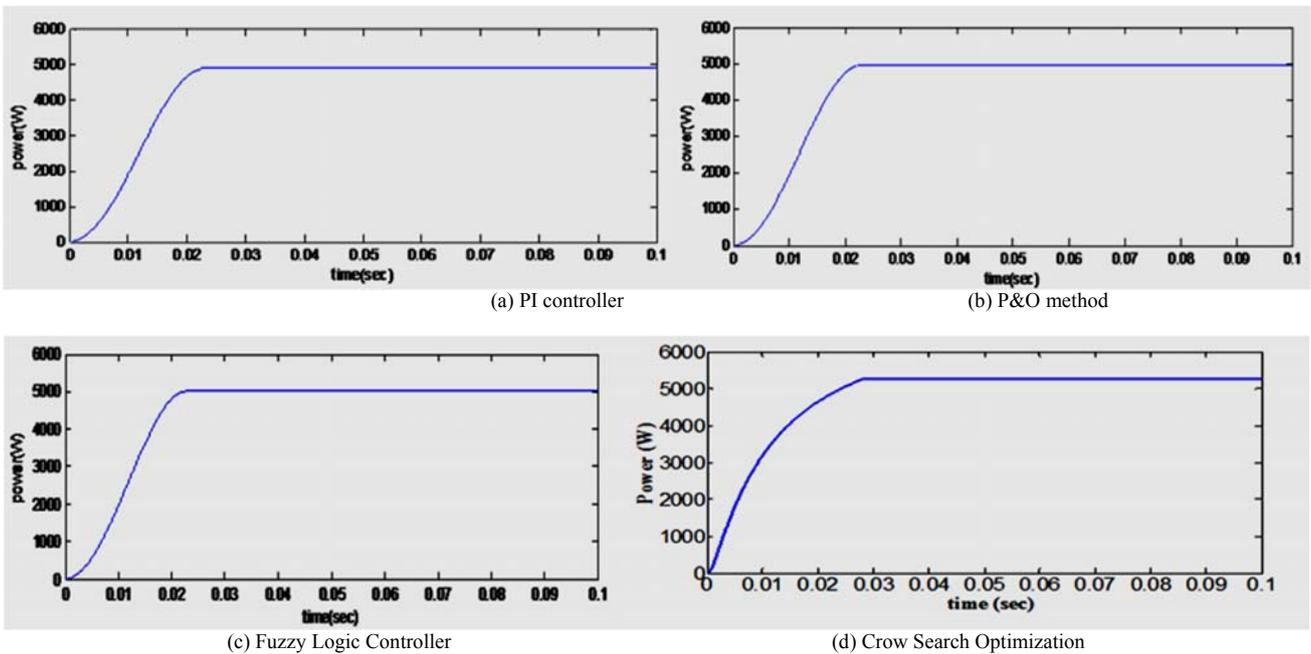
Fig. 5. Power obtained by different MPPT techniques
