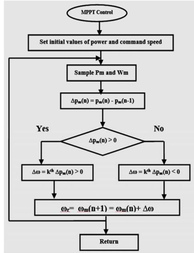
Fig 2. Flow chart for MPPT controller
