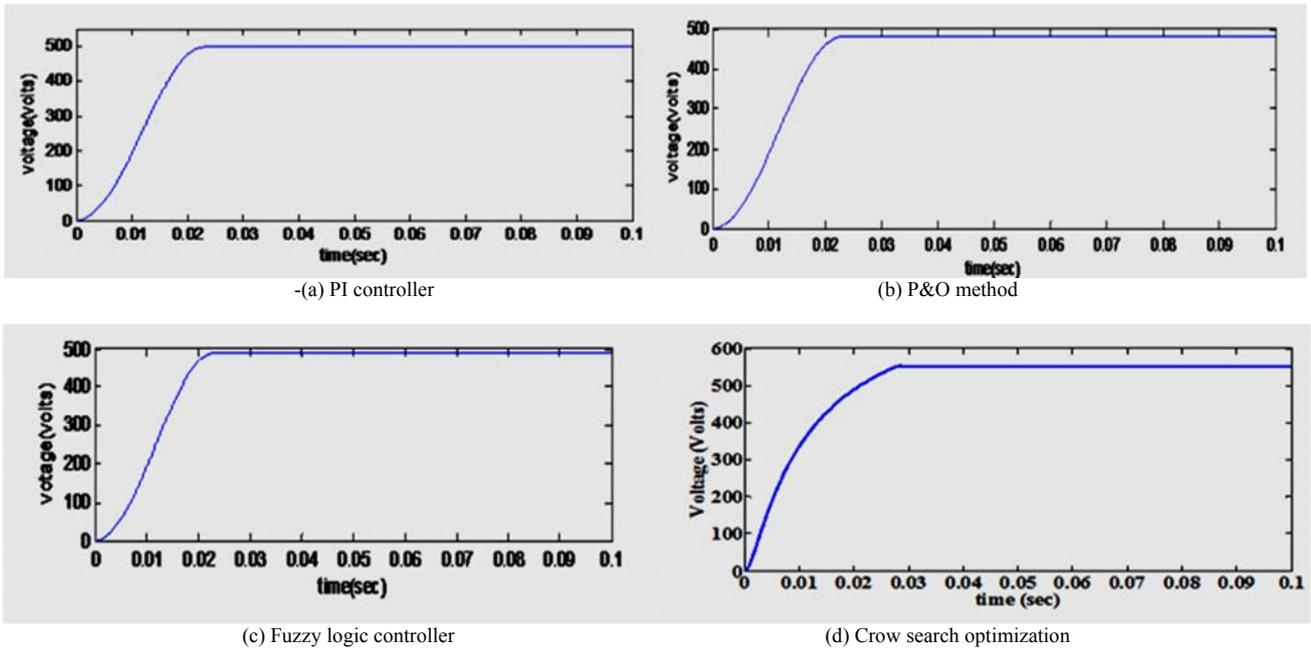
Fig. 4. Output voltage comparison of MPPT techniques
