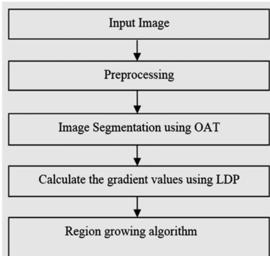
Figure 1: Proposed titanium-coated surface crack detection system
