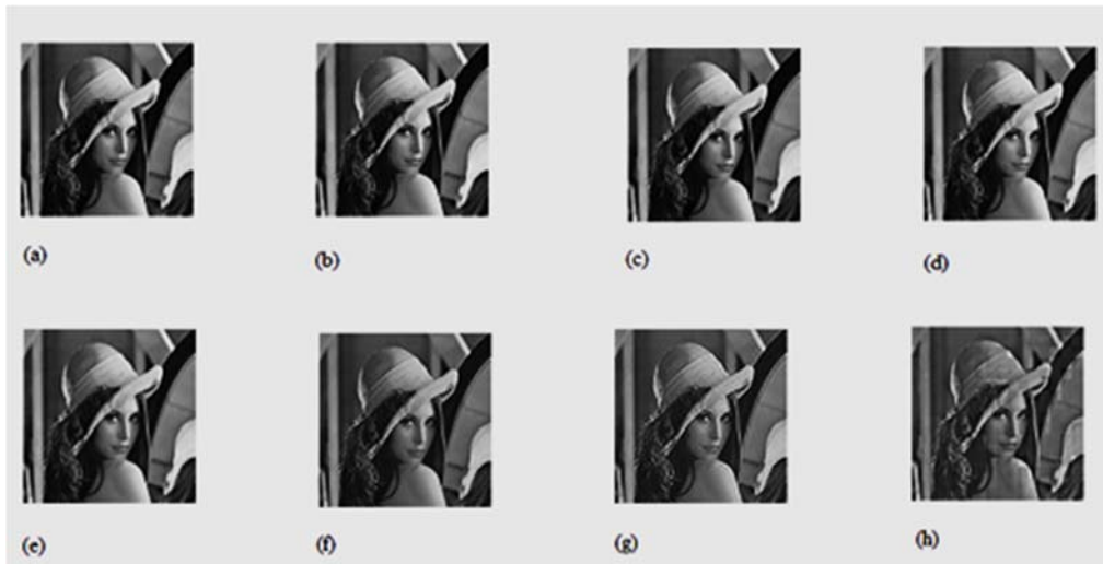
Fig. 6. Watermarked images with Algorithm 2 for different embedding rate: (a) 1/64 bpp (b) 1/32 bpp (c) 1/16 bpp (d) 1/8 bpp (e) 1/4 bpp (f) 1/2 bpp (g) 3/4 bpp (h) 63/64 bpp
