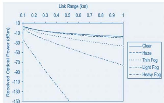
Fig 10. Link range versus Received optical power for 1550 nm transmission
