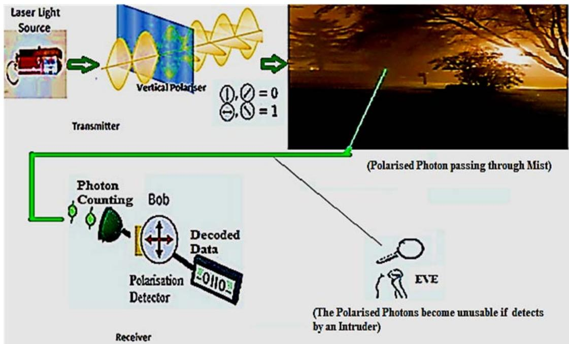
Fig 8 .Quantum key distributions through Misty and Fog environment.
