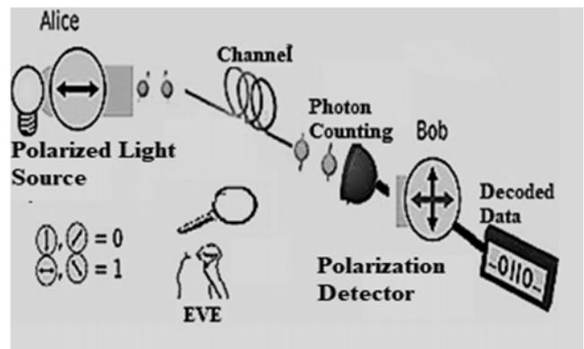
Fig 5. Quantum Key Distribution System
