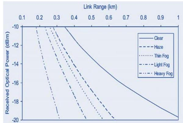
Fig 9. Link range versus Received optical power for 785 nm transmission
