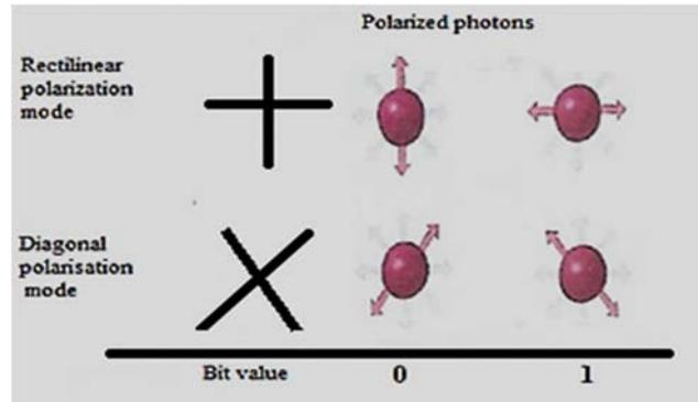
Fig 2. Polarized photons and corresponding bit values.
