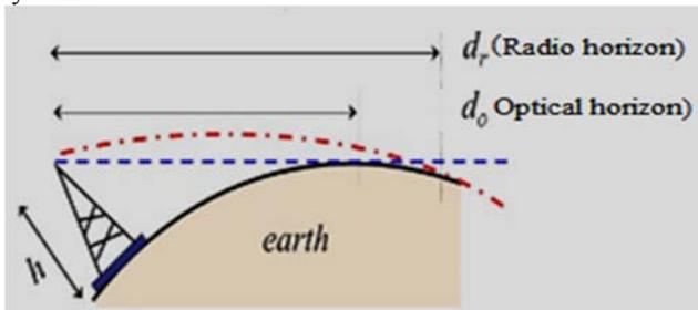
Fig 4. Optical and Radio Horizon
