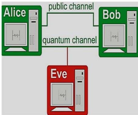
Fig 1. Simplified Quantum key distribution
