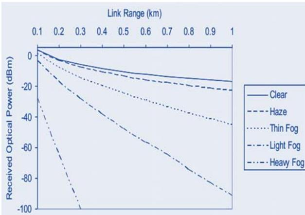
Fig 11. Link range versus Received optical power for 650 nm transmission
