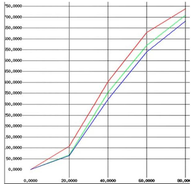
Fig 5: Packet delay among various routing protocols: Red=LEACH-MA-delay, Green=MACO-delay, Blue=EMRP-AIPUR-delay
