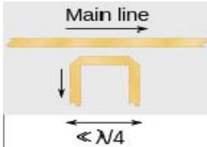
Figure 3 Short section directional coupler
