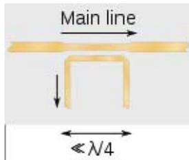
Figure 4 Short section directional coupler with 50 Ω main line and 100 Ω coupled line
