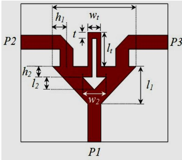
Figure 8. Geometry of proposed TPD Design-top view.
