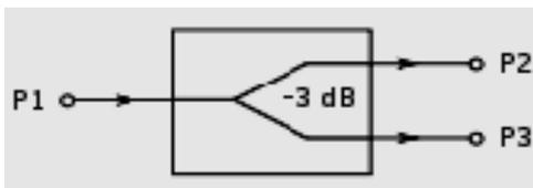
Figure 1. Symbol for power divider
