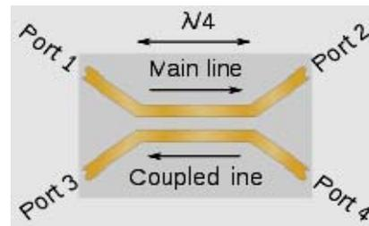
Figure 2. Single section  $\lambda/4$  directional coupler
