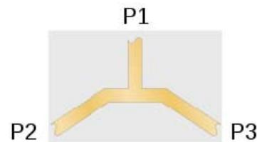
Figure. 5-b Simple T-junction power division in planar format
