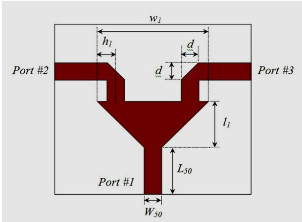
Figure 6. Triangular Shaped Wilkinson Power Divider
