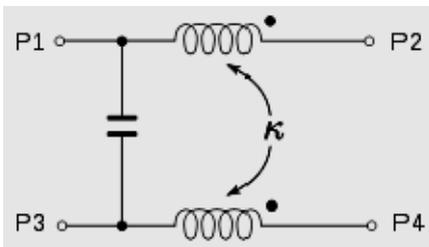
Figure 5-a. Lumped element equivalent circuit of the couplers
