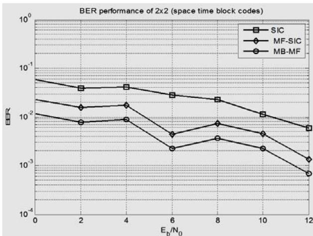
Fig 4. BER performance of 2x2 Antenna system
