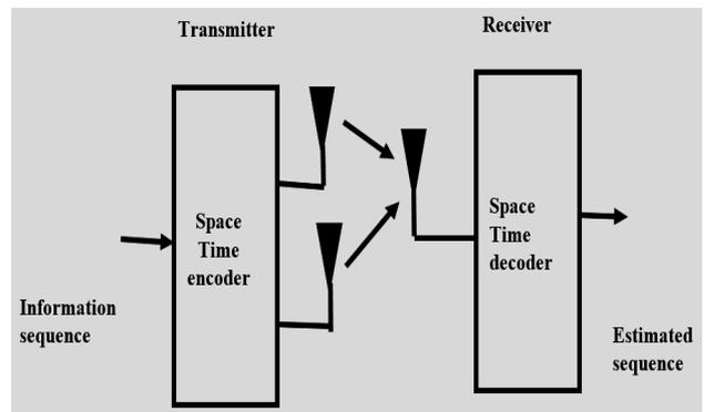
Fig 2. Basic Structure of Space Time Coding
