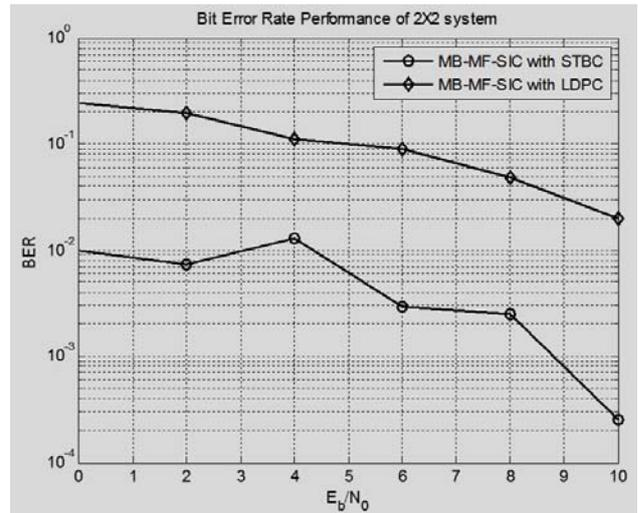
Fig 5. Bit Error rate Performance of STBC and LDPC of 2x2 system
