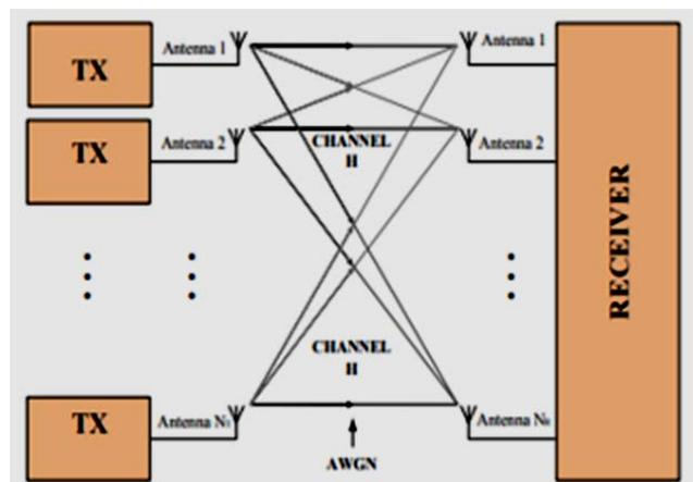
Fig 1. Multiple Input Multiple Output system.
