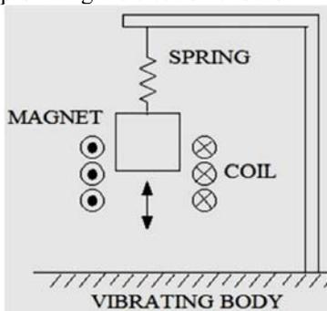
Fig.2 Diagram of electromagnetic micro generator
