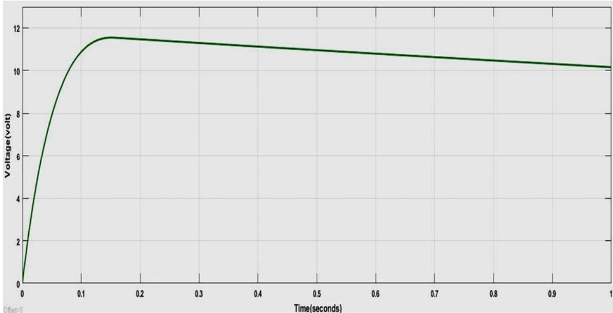
Figure 10 shows the obtained output voltage of the ac to dc converter ranges from 9V-12V when the person is running condition.
