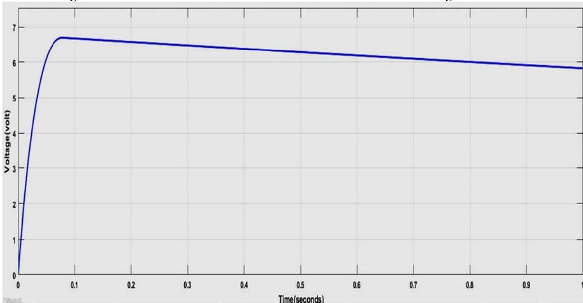
Figure 11 shows the obtained output voltage of the ac to dc converter ranges from 2V-12V when the person is jumping condition.
