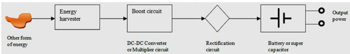
Fig 4. Basic design of Energy Harvesting System.
