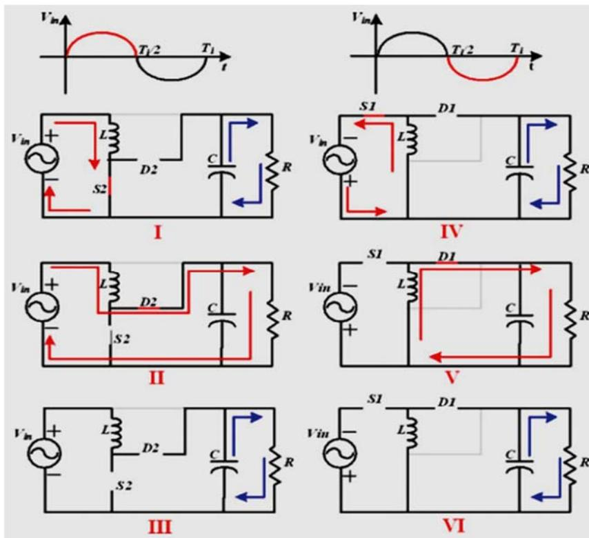
Fig.6 Operation modes of the proposed AC-DC converter
