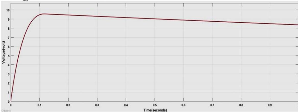
Figure 8 shows the obtained output voltage of ac to dc converter ranges from 8V-10V when the person is cycling condition.
