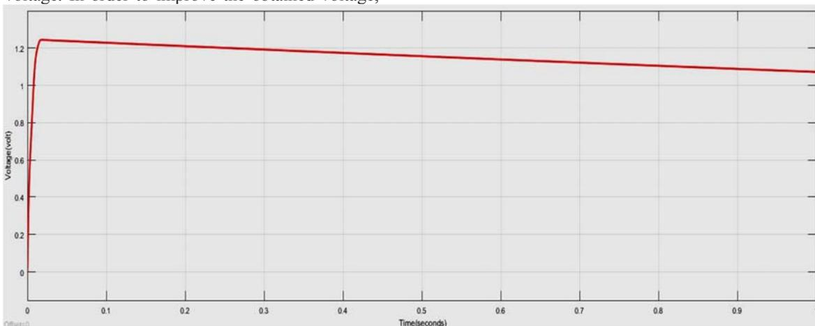
Figure 9 shows the obtained output voltage of the ac to dc converter ranges from 0.8V-1.5V when the person is cycling condition.
