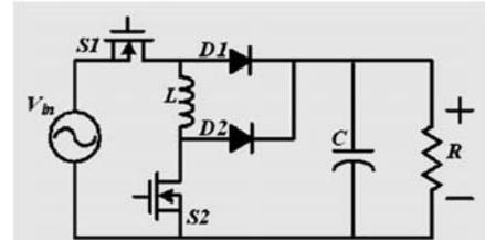
Fig.3 Bridgeless boost rectifier for energy harvest
