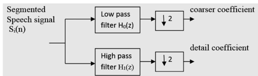
Fig 2.1 Decomposed structure of DWT
