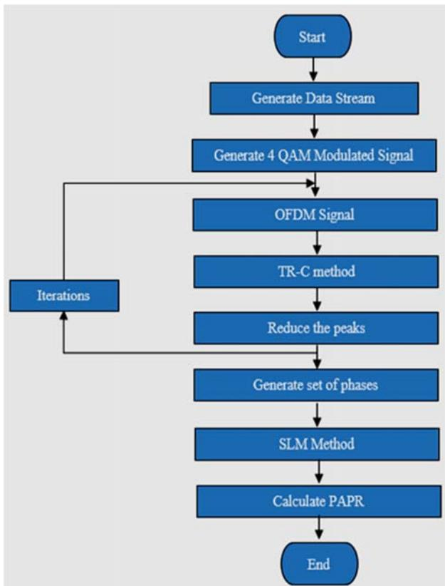
Figure 3. TR-C+SLM flowchart
