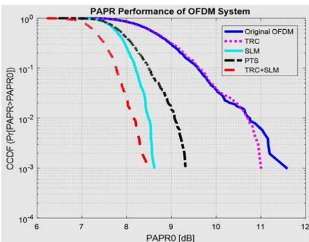
Figure 7. Original OFDM, TRC, SLM, PTS Vs and combined TRC SLM Technique under 4 QAM condition and N=1024
