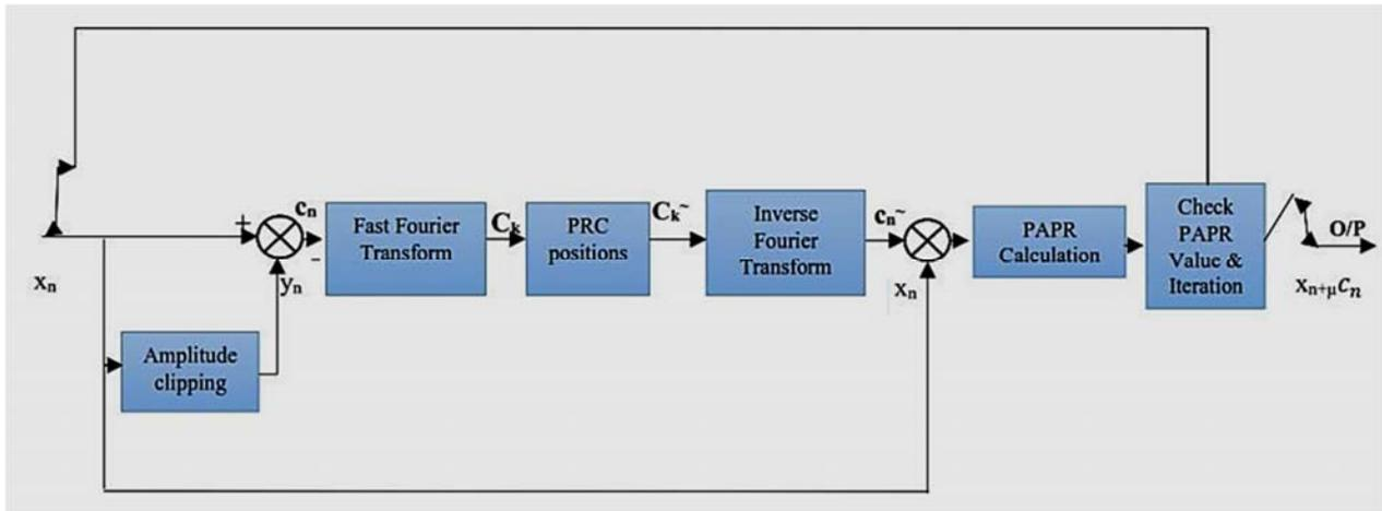
Figure 2. Block diagram of the clipping based TR [14]
