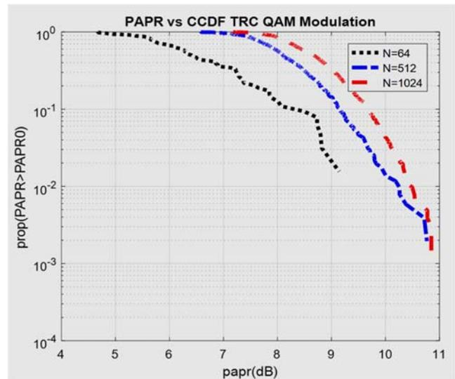
Figure 4. TRC method for QAM OFDM method with different number of subcarriers
