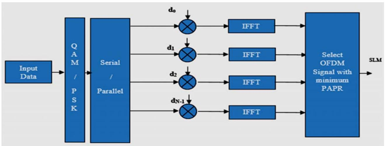
Figure 1. SLM Technique block diagram
