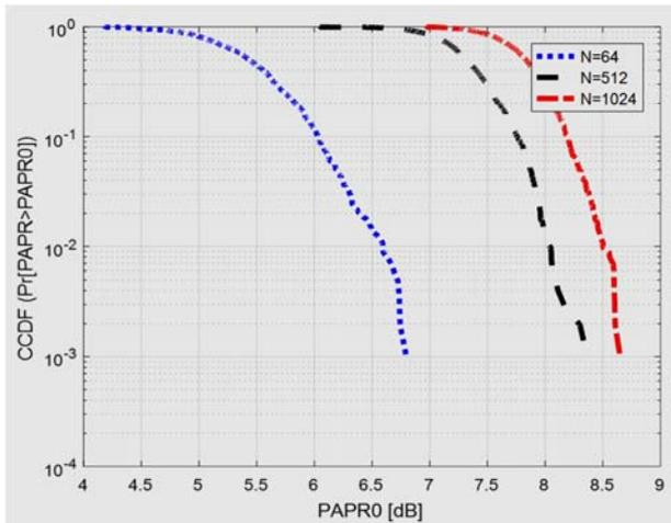
Figure 5. SLM Method for QAM OFDM System with different number of subcarriers
