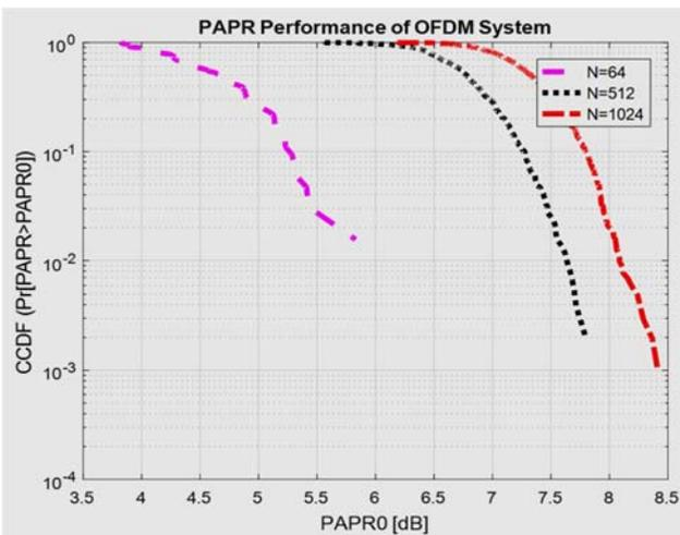
Figure 6. TRC-SLM Combined method for 4QAM OFDM System with different number of subcarriers
