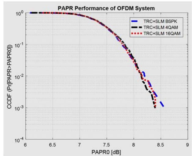
Figure 8. TRC-SLM performance for different modulation schemes
