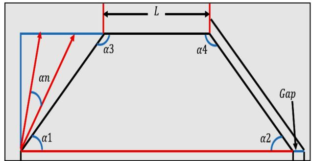
Fig. 4. The dimensions of the T-joint section with parameter effect
