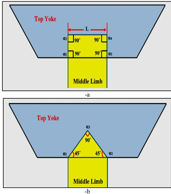
Fig. 3 Description of T-joint designs (a) 90° butt-lap (b) 45° mitered
