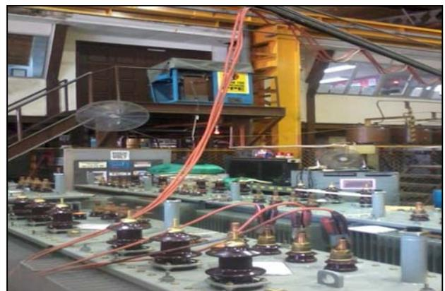
Fig. 9. The experimental test for transformer type butt-lap T-joint design
