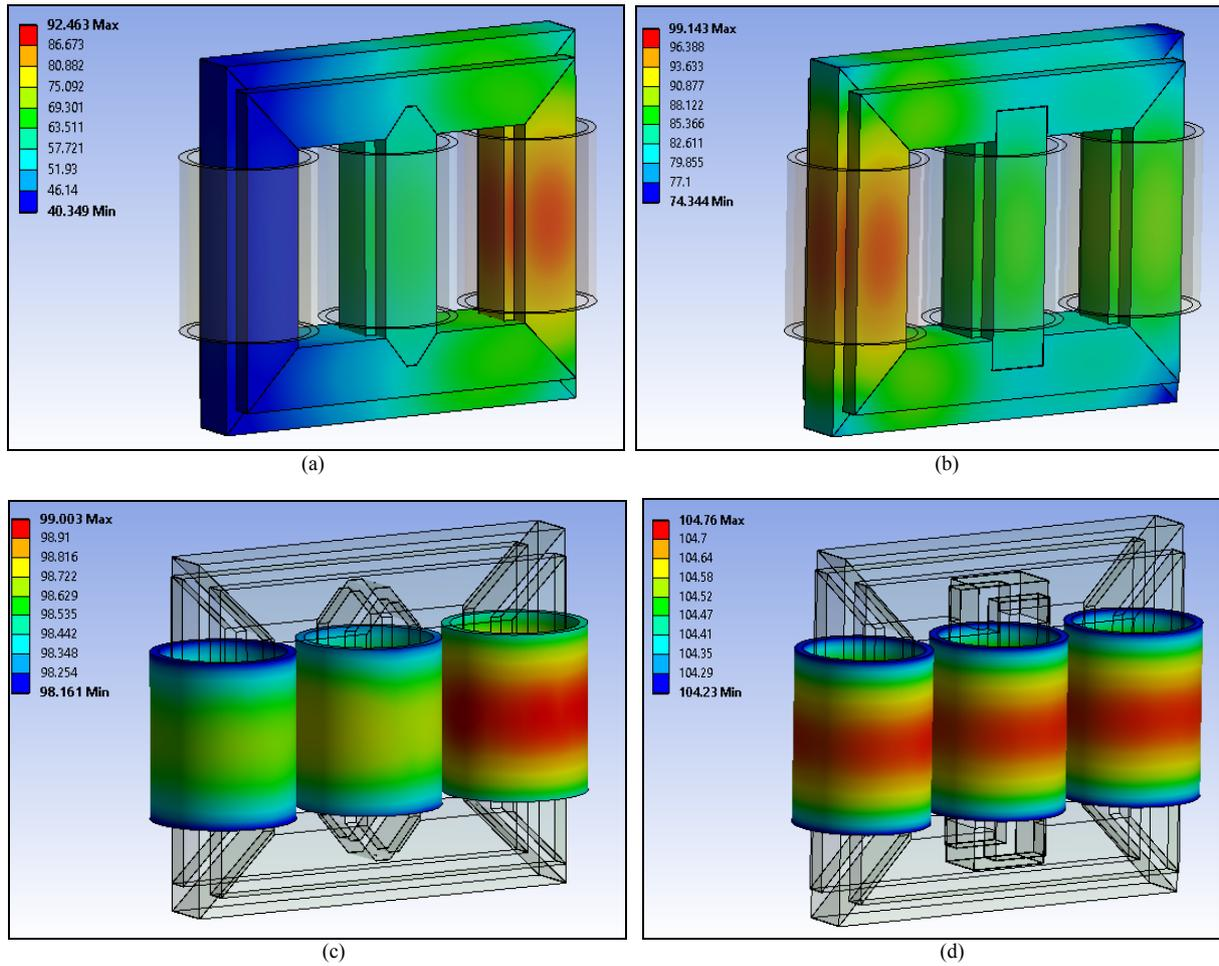
Fig. 8. The core and windings temperature on the full load for different designs of T-joints (a) proposed design (b) butt-lap core (c) windings in proposed design (d) windings in butt-lap
