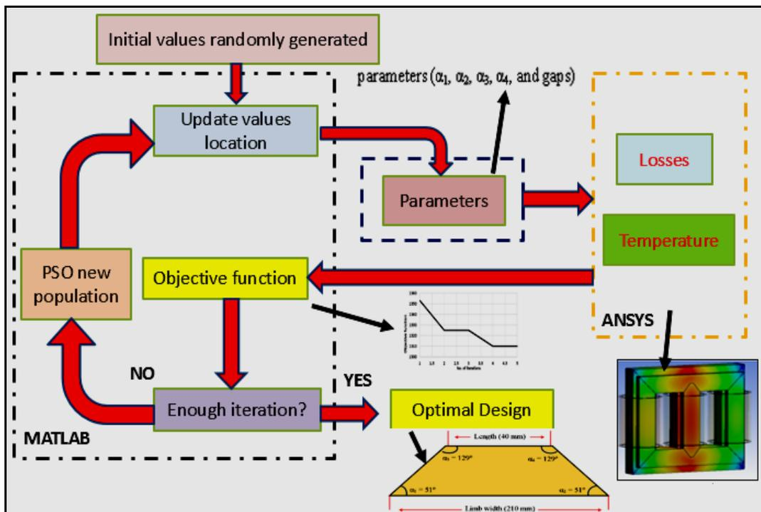
Fig. 5 The interaction between Mat lab with ANSYS software
