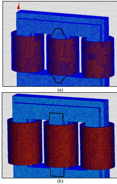
Fig. 2 3D Model mesh analysis in ANSYS Software (a)proposed design (b) 90° butt-lap design
