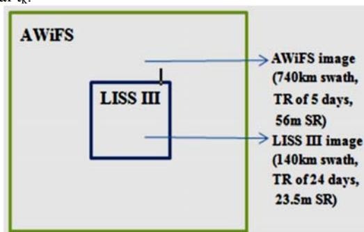
Figure 1. Cross Section of LISS-III and AWiFS
