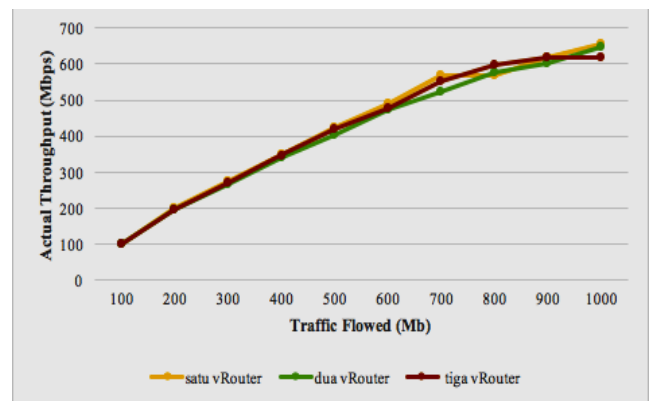
Fig. 13. Graph of UDP throughput testing results on the number of routers
