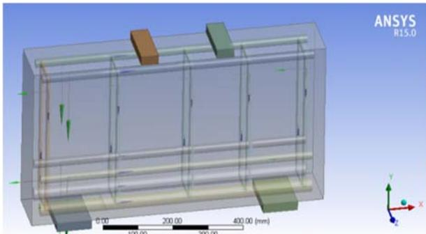
Fig.4. Reinforced Cement Concrete (of grade M40) deep beam modeled in ANSYS R15.0
