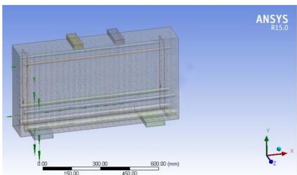
Fig.5. Fibre Reinforced Engineered Cementitious Composite (of grade M40) deep beam modeled in ANSYS R15.0
