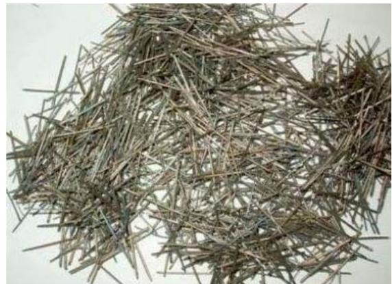
Fig.2.Steel Fibers used in ECC
