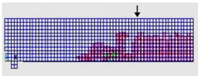
Fig.7. Crack simulation in RC Deep beam in half the span
