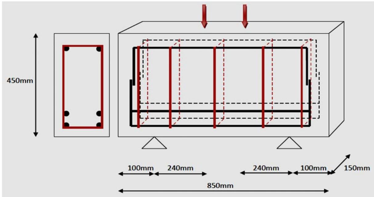
Fig.3. Deep beam section details being modeled as CC and ECC of M40 grade.
