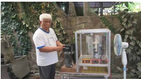
Fig. 7. The Microcontroller, wind tunnel and VAWT
