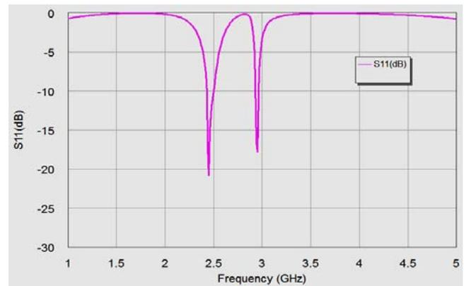
Figure 2. S11 response of the microstrip quasi-fractal antenna
