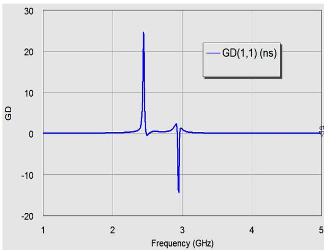
Figure 4. The group delay response of the microstrip antenna
