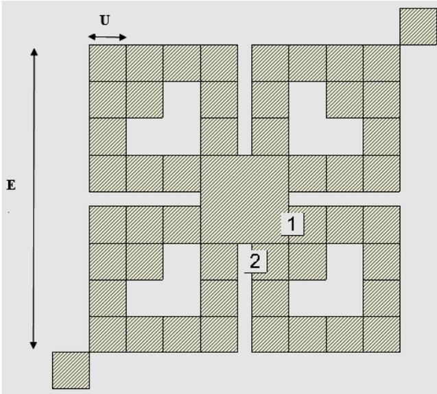
Figure 1. The top view topology of quasi-fractal antenna.
