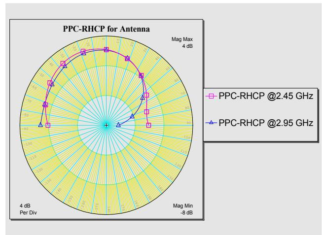
Figure 6. PPC-RHCP radiation results for quasi fractal antenna
