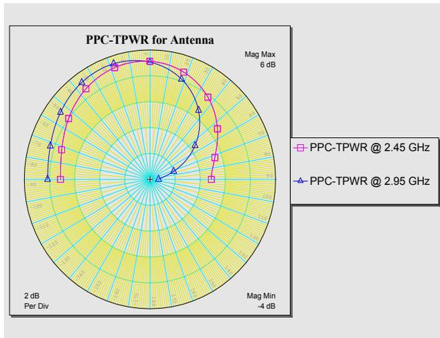
Figure 7. PPC-TPWR radiation results for quasi fractal antenna
