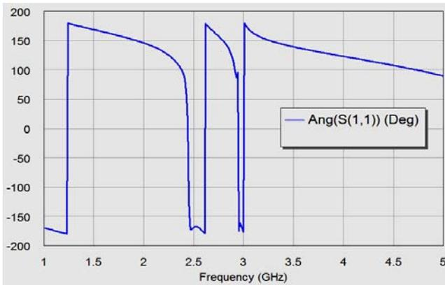
Figure 3. The phase response of the microstrip quasi-fractal antenna
