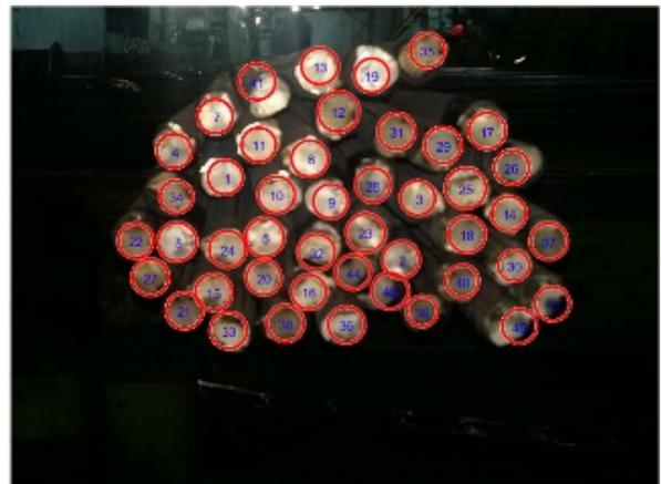
Figure 13. Detecting Round Objects Using Hough Transform
