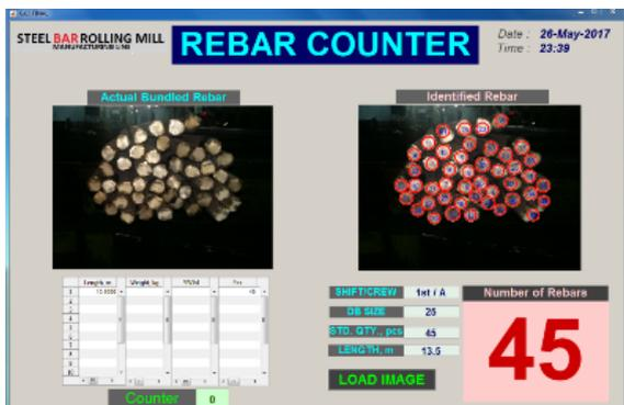
Figure 16. GUI showing the output quantity of the system and the standard quantity
