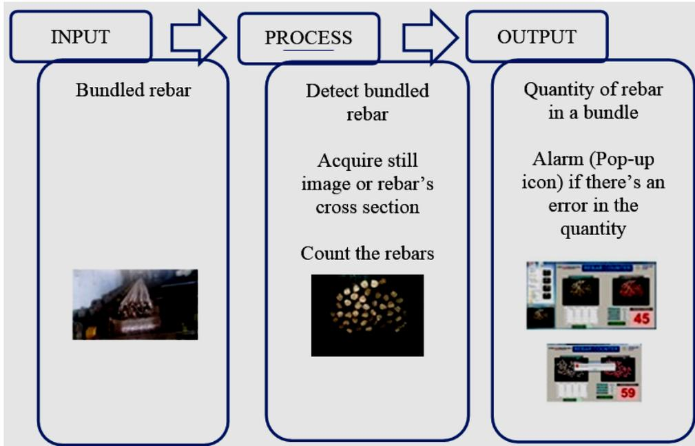
Figure 1. Rebar Counter’s Conceptual Framework
