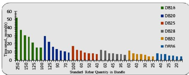
Figure 17. Increasing Time Saved as Quantity of Rebar Increases
