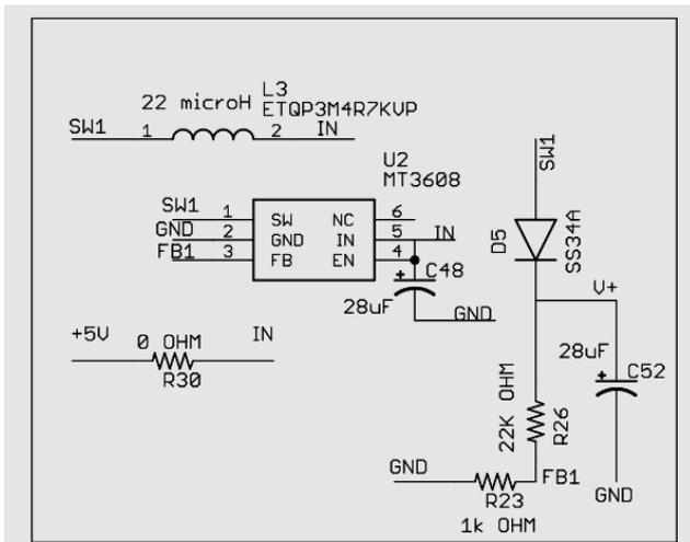
Figure 4. Switching Regulator for +14 Volts
