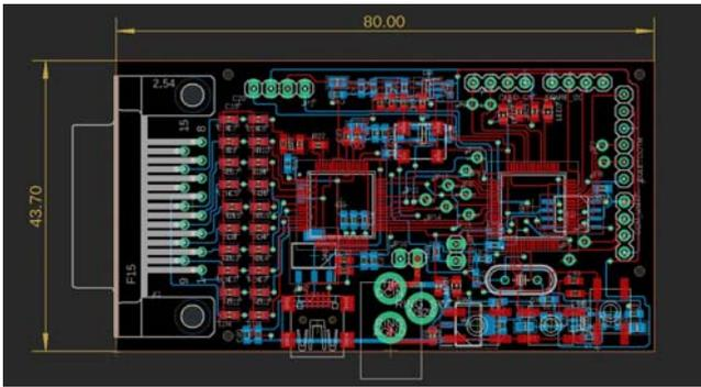
Figure 7. PCB layout for Design 2
