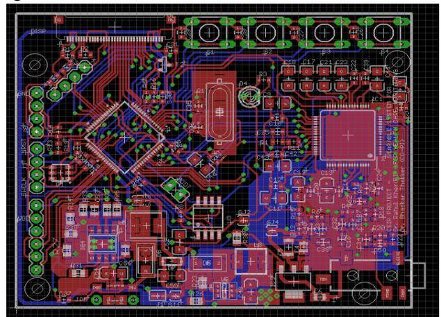
Figure 5. Double side PCB layout for Design 1
