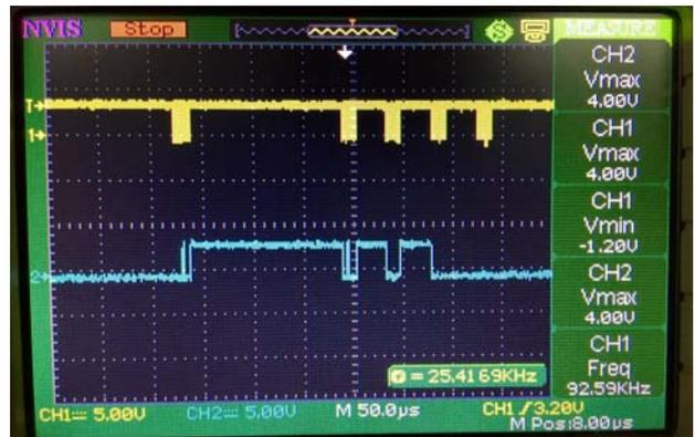
Figure 9. Image of all SPI signals transmitted
