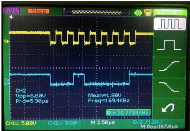
Figure 11. Transmission of RREG signal byte 1 (0x21)
