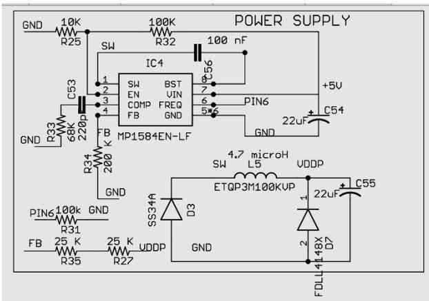
Figure 3. Switching Regulator for +3.3 Volts
