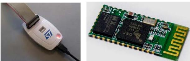
Figure 2. ST-Link/V2 In-circuit Debugger; HC 05 Bluetooth module
