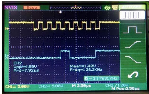
Figure 10. Image of transmission of SDATAC signal (0x11)
