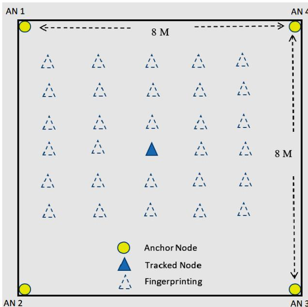
Figure 3. RSS Fingerprint position for 30 different locations.
