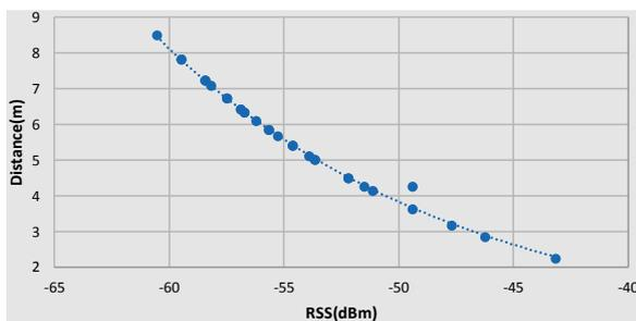
A. Comparison of RSSI to distance on anchor node 1
