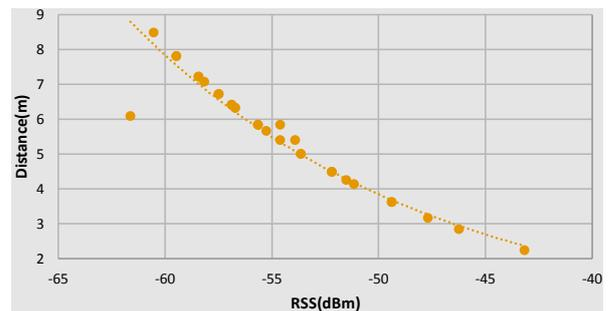
D. Comparison of RSSI to distance on anchor node 4
