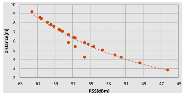
B. Comparison of RSSI to distance on anchor node 2
