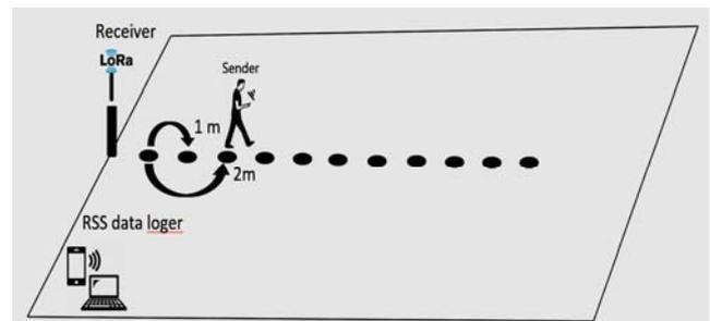
Figure 4. RSS measurement position testbed in interval 1 m and 2m.
