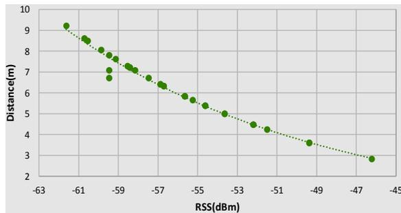
C. Comparison of RSSI to distance on anchor node 3
