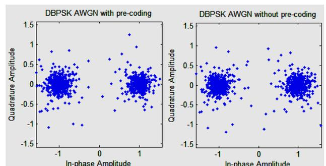
Fig.06. Simulated DBPSK Constellations for the Rician Distribution.
