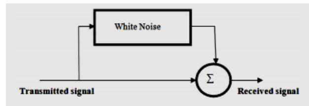
Fig.01. Representation of AWGN channel
