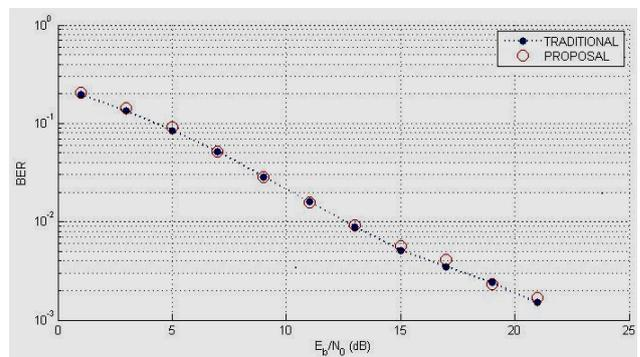
Fig. 09. BER between the models for Rician fading.
