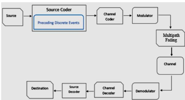
Fig.04. Wireless Model with the Proposal of this study
