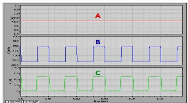
Figure 7. Simulation result of the current sensing circuit, (A) output voltage, (B) sensing signal, and (C) inductor voltage  $V_x$ .
