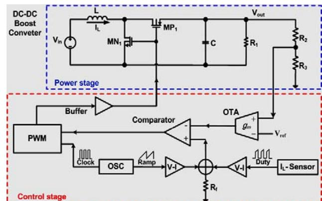
Figure 1. The block diagram of a current-mode boost converter.
