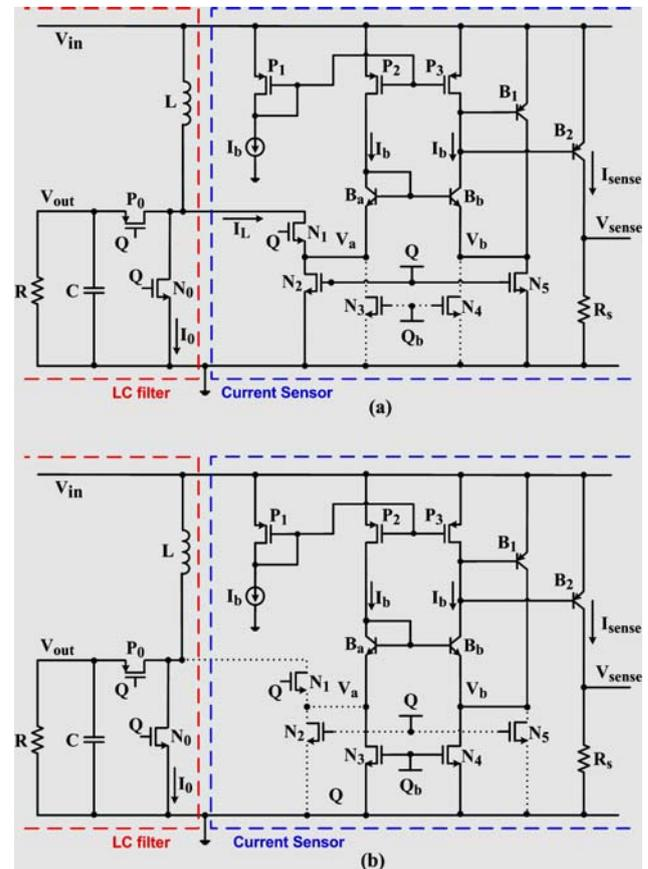
Figure 4. Current-sensing circuit during the (a) ON period and (b) OFF period.
