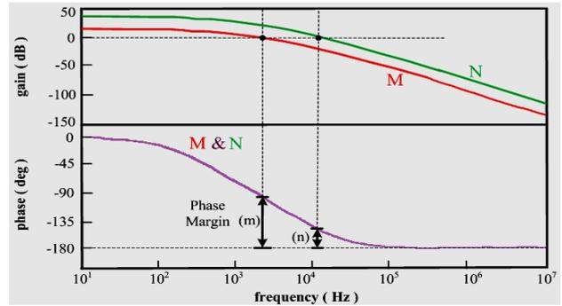
Figure 6. Frequency response of the output of error amplifier with the difference of the gain in amplifier, (M)  $16\ \text{dB}$  and (N)  $37\ \text{dB}$ .
