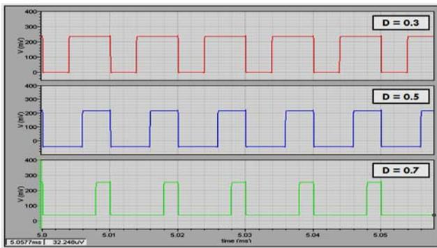
Figure 8. Simulation result of the sensing signals with the duty ratio of 0.3, 0.5 and 0.7.
