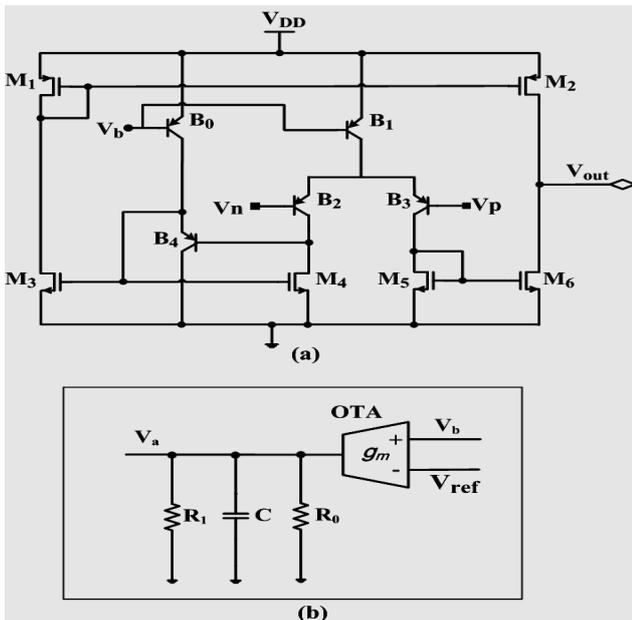
Figure 2. Schematic of (a) OTA circuit with (b) compensator circuit.
