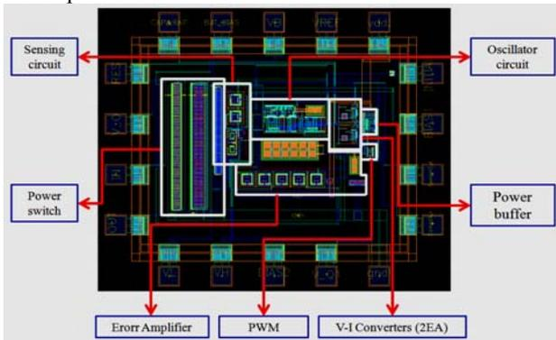
Figure 5. Layout of DC-DC boost converter.
