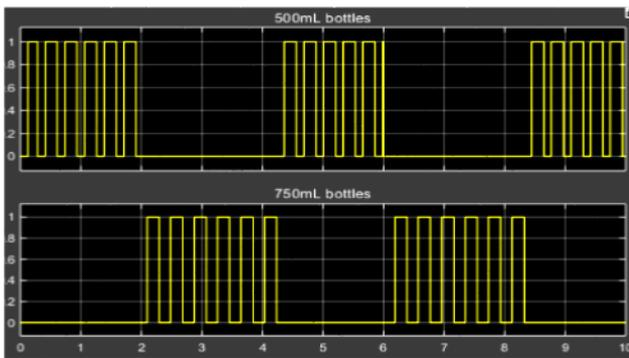
Figure 4. Simulated output of water filling subsystem showing the 500 ml and 750 ml bottles.
