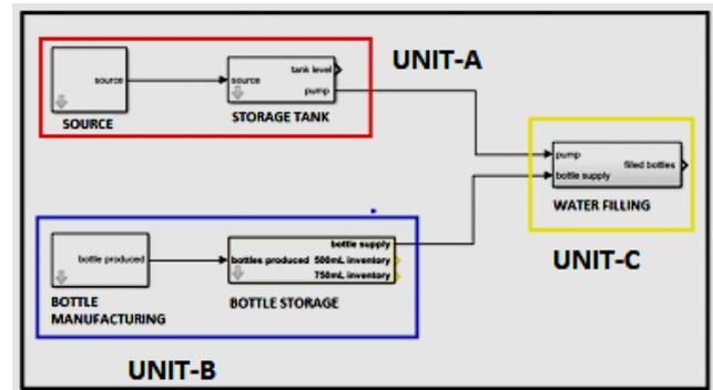
Figure 2. Simulink model for the plant showing three main units
