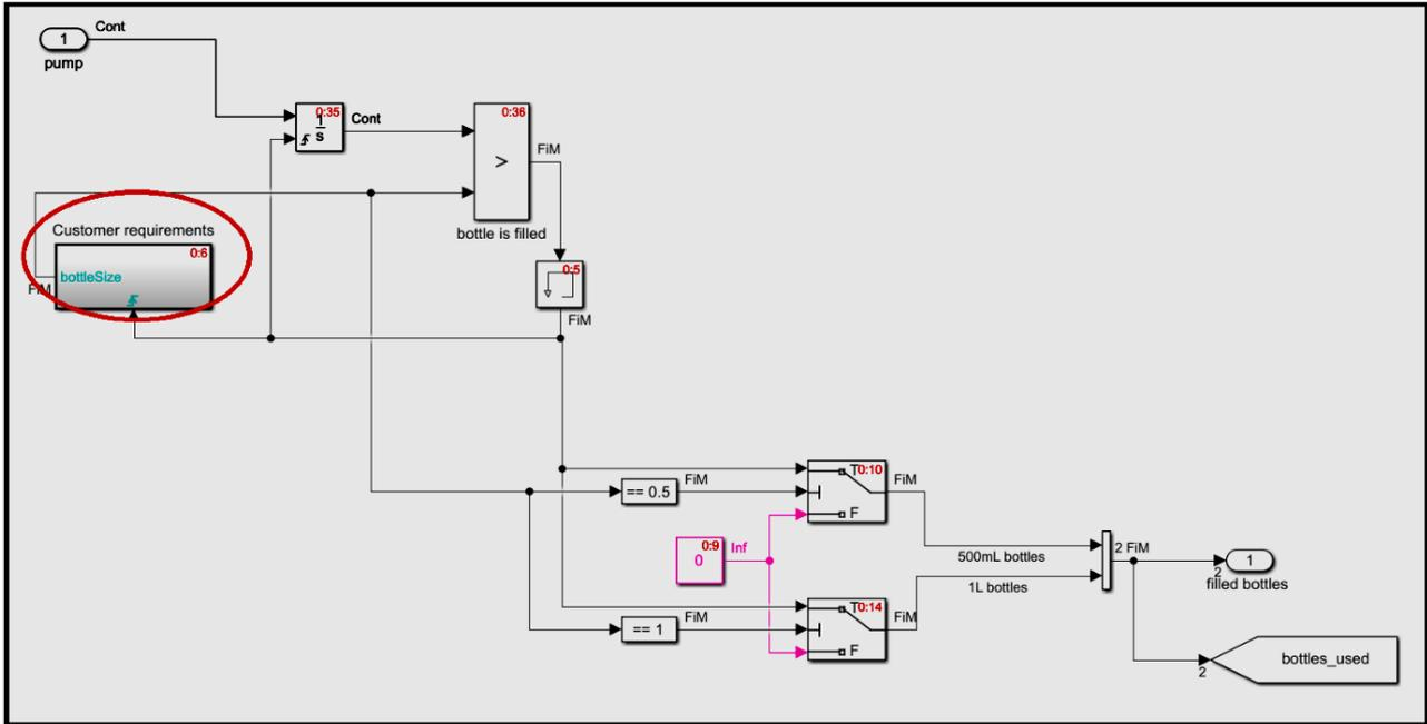
Figure 5. Water filling unit with customer requirements subsystem
