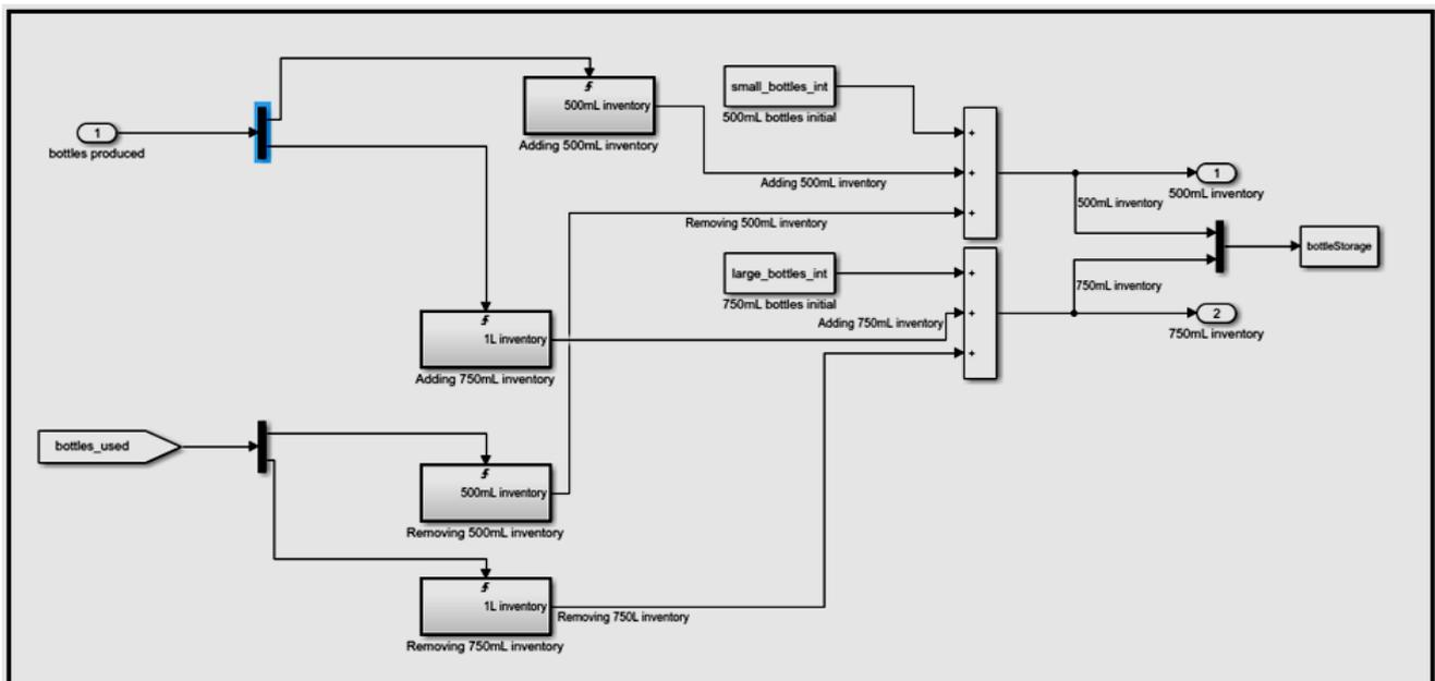
Figure 3. Bottle storage subsystem
