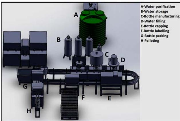
Figure 1. A 3dimensional CAD model of the plant
