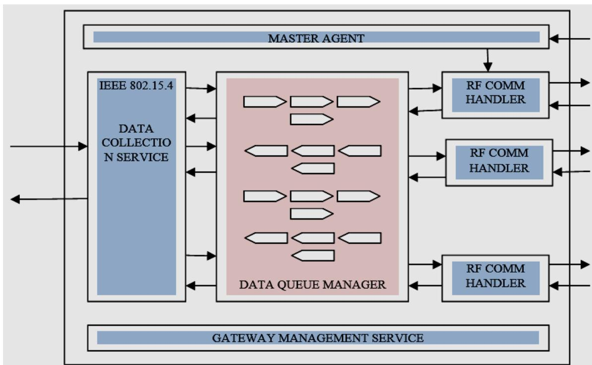
Fig.3. Gateway Software Architecture
