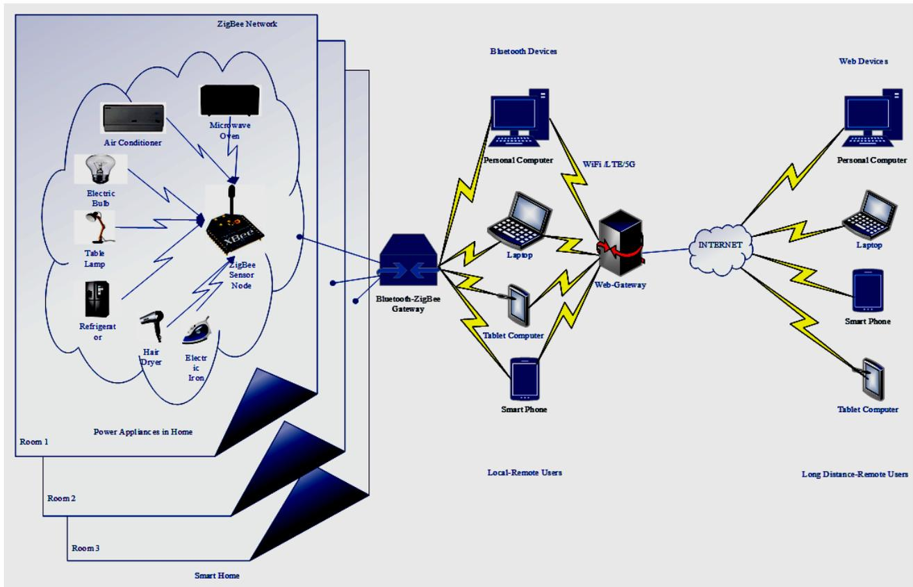
Fig.1. Conceptual Overview of Smart Home through Bluetooth-ZigBee Gateway
