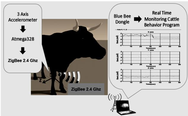
Figure 2. Device installation and accelerometer sensor.
