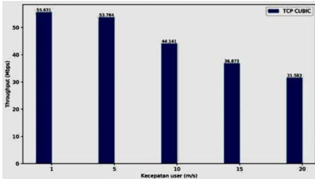
Fig. 5. TCP CUBICs Throughput on Dual Connectivity Handover.
