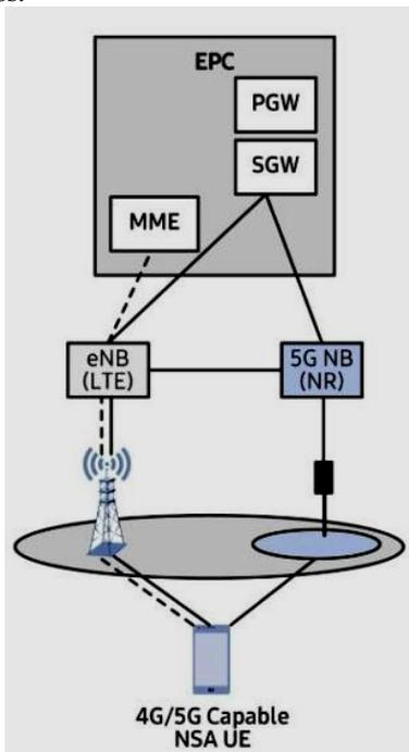
Fig. 2. Handover Dual Connectivity System [7]
