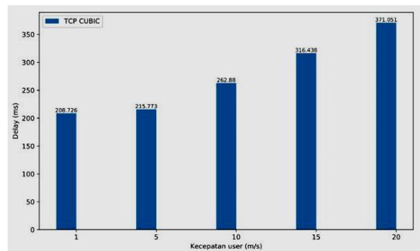
Fig. 4. TCP CUBICs Delay on Dual Connectivity Handover.
