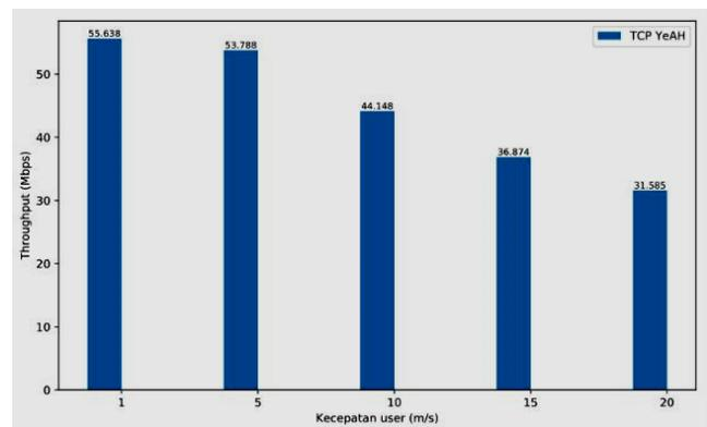
Fig. 7. TCP YeAh's Throughput on Dual Connectivity Handover.
