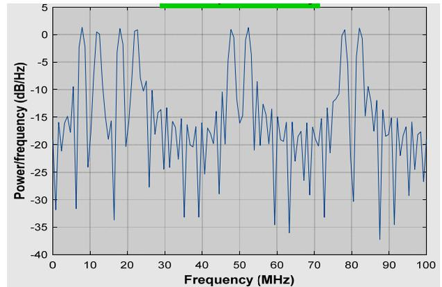
Fig. 8. Power Spectral Density at attenuation of received signal by 30%
