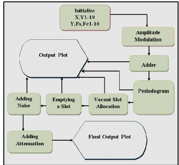
Fig. 3. Block Diagram of Cognitive Radio System
