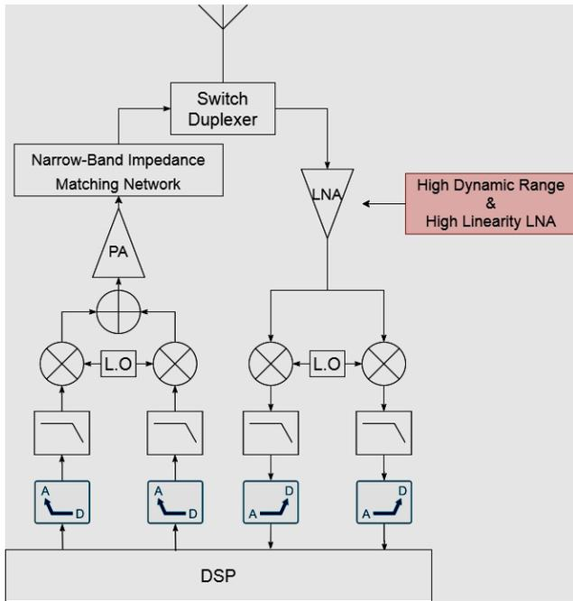
Fig. 2. CR transceiver architectures [22]
