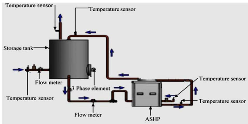
Figure 2. Schematic diagram of the electric boiler retrofitted with an ASHP unit.
