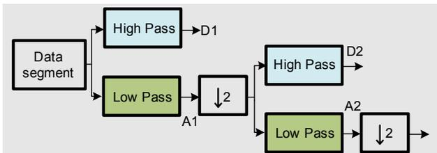
Fig. 2. Two-level wavelet tree decomposition where the framed signal is fed into a high pass and low pass filter to yield the detail and approximation coefficients respectively. The approximation coefficients are then down-sampled by two before the decomposition is repeated again to give the coefficients at the subsequent level.
