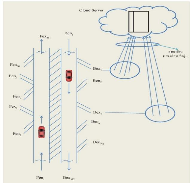
Figure 1. A model of the intercity motorway showing the entrance points, and exit points. The information of each of these points consists of name, GPS location. The horse-shoe U-turn, and the exit-entrance U-turn [1].
