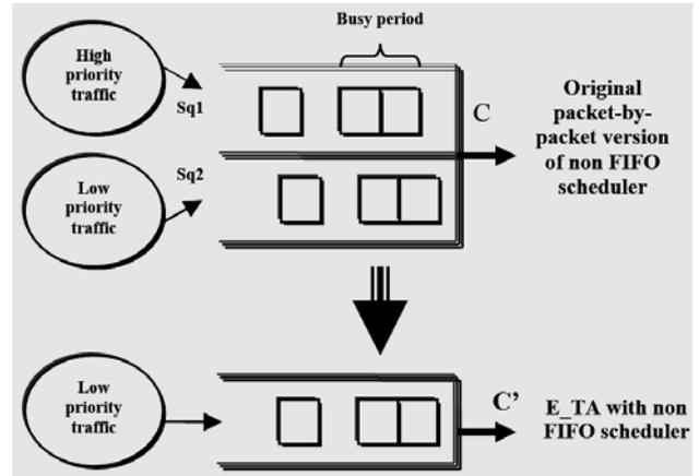
Figure 2. The elimination of sq1 in E\_TA accelerated simulation technique
