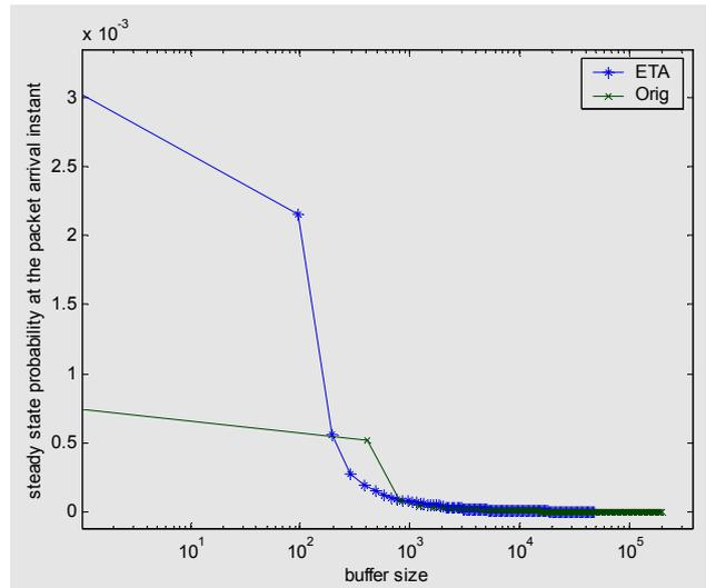
Figure 4: The queuing distribution in sq2 of the non FIFO scheduler for E\_TA with non FIFO scheduler (ETA) and original packet-by-packet model (orig)
