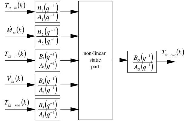
Figure 3: The Wiener-Hammerstein cascade model for the superheater
