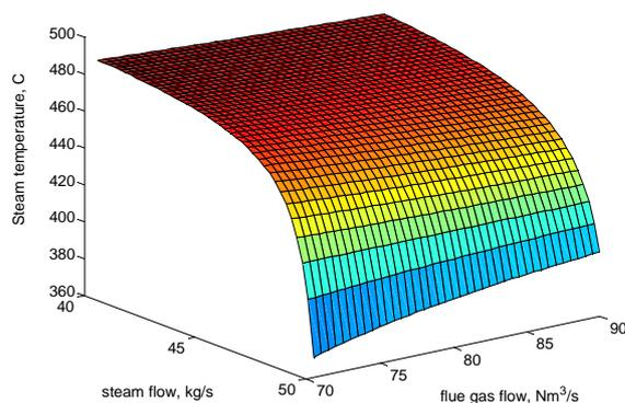
**Figure 8:** The steady state characteristic: the superheated steam temperature as a function of the steam and fuel flow.
