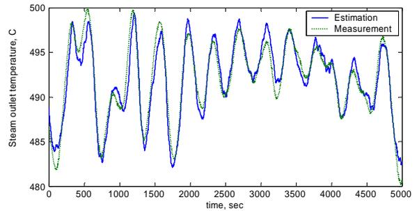
Figure 6: The measured and estimated outlet steam temperature in the validation
