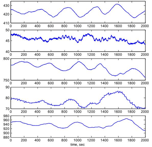
Figure 5: The model input variables (steam inlet temperature, steam mass flow, flue gas inlet temperature, flue gas volume flow, flue-gas representative temperature in the combustion chamber respectively) on the time range applied in the identification
