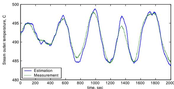
Figure 4: The measured and estimated outlet steam temperature in the identification
