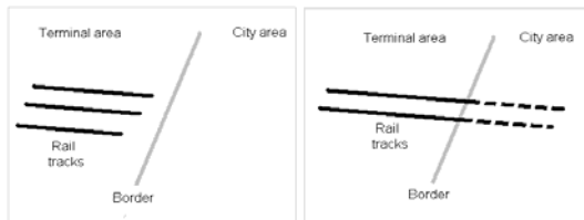
Figure 4: Differences between conceptions of length improvements of rail tracks
