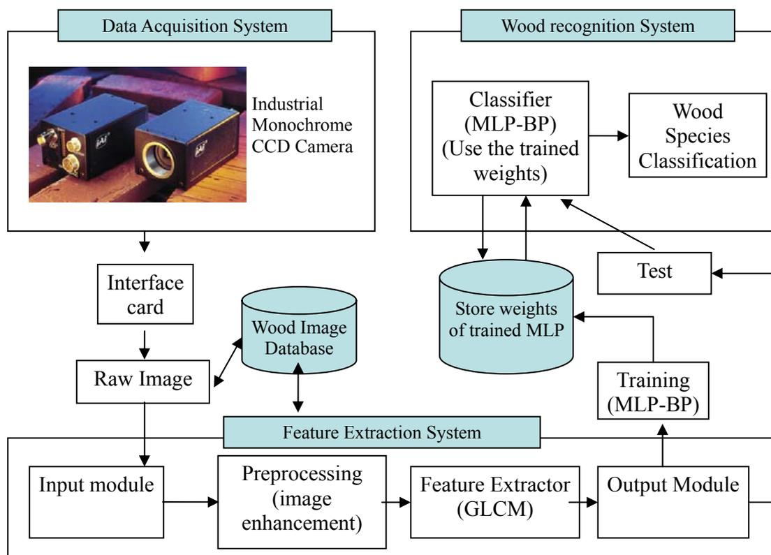
Fig. 2. A block diagram showing the procedures of the wood recognition system.
