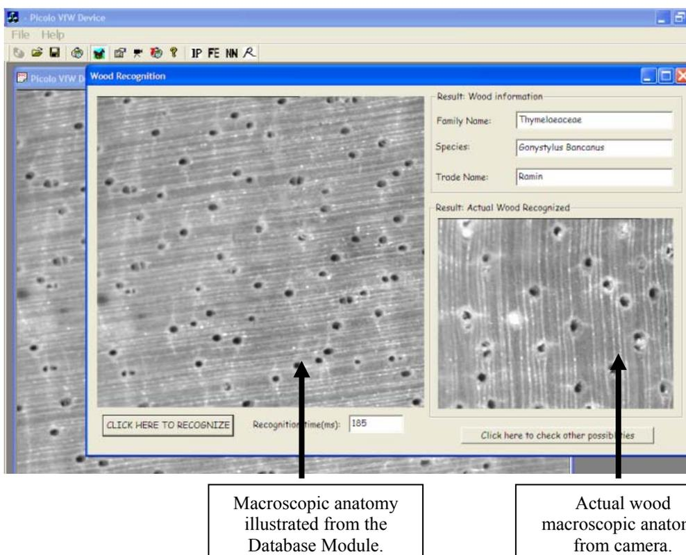
Fig. 8. Example of the results given by the Recognition Module of the Wood Recognition System.
