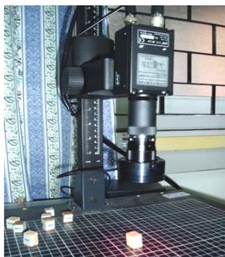
Fig 3. A CCD camera with a 40mm extension tube is used to acquire the macroscopic wood anatomy.
