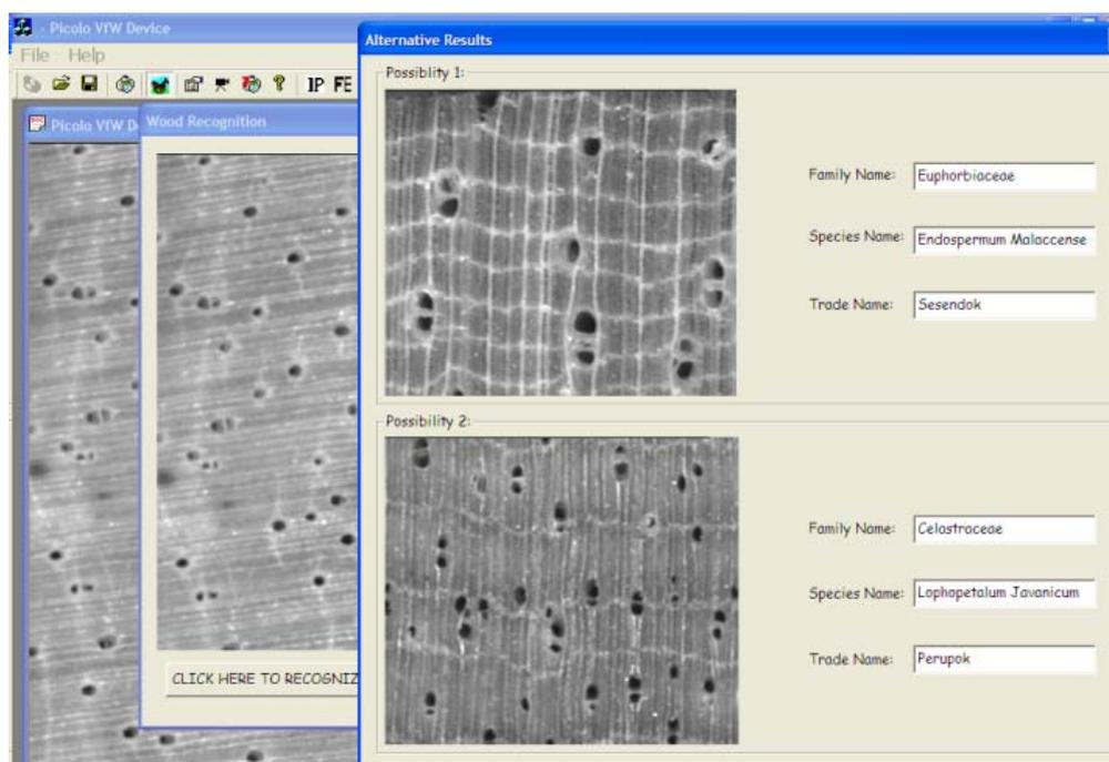
Fig. 9. Example showing two other alternative answers together with illustrations of their respective macroscopic anatomies given by the Recognition Module of the Wood Recognition System.
