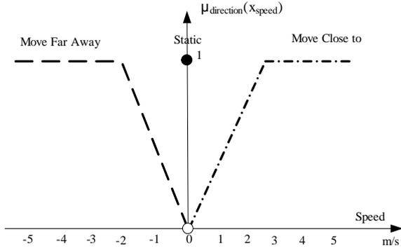
Figure 9 Fuzzy Conversion Scale for MN's Moving Direction Relative to BSs
