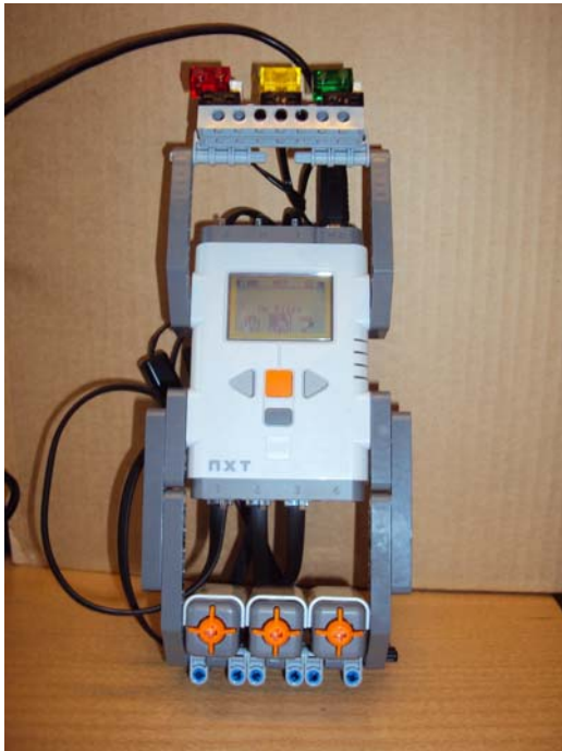
Fig. 10: LEGO Mindstorms robot setup as a traffic lights simulator
