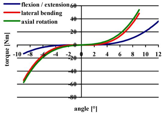
Figure 3. Characteristic curve torque-angle L3-L2.
