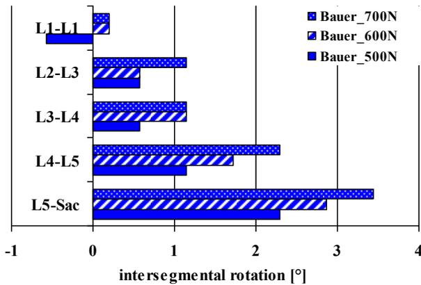
Figure 12. Intersegmental rotation of the FSU's under different loads.
