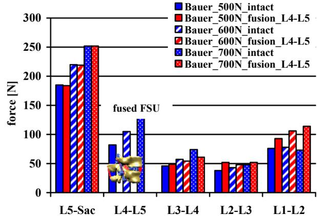
Figure 14. Comparison of the facet forces of model 1 and model 2 during different loads.
