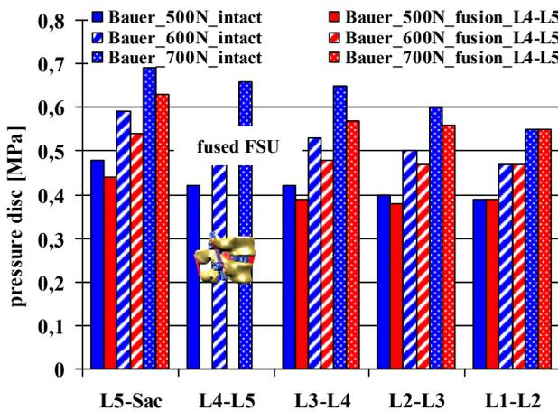
Figure 13. Comparison of the intradiscal pressure of model 1 and model 2 during different loads.
