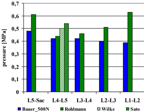
Figure 8. Comparison of the model simulation results with FE-Model and in vivo experiments of the disc pressure.
