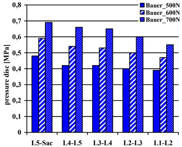
Figure 10. Comparison of the pressure in the discs of model 1 during different loads.
