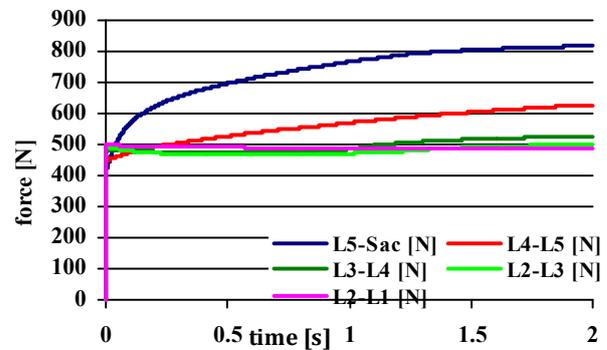
Figure 6. Reaction forces of the discs in vertical direction of the different functional units during an acting force of 500N.
