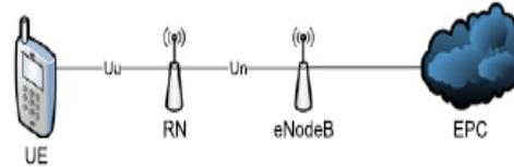
Figure 3 Relay basic scheme
