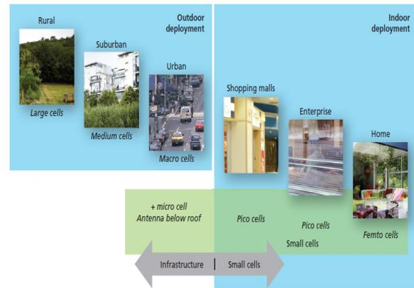
Figure 2 Radio propagation environments
