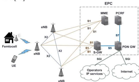
Figure 1 network architecture of LTE-Advanced
